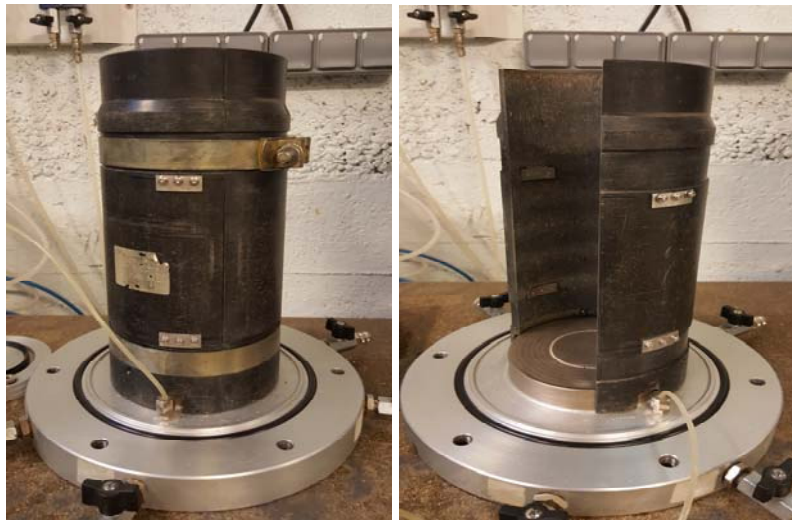
Figure A.3. Photos of the fixing devices for the displacement transducers on the compaction mould
