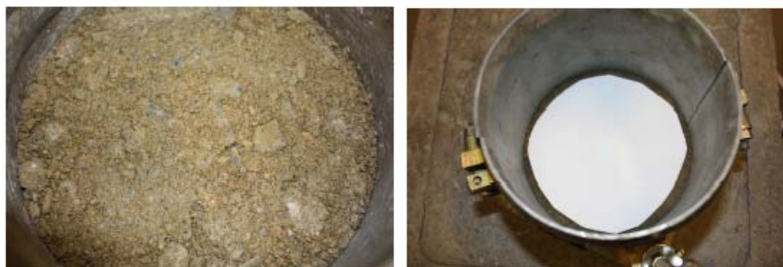
Figure II.11. Filter paper inserted in a sample of UGM Maraîchères
