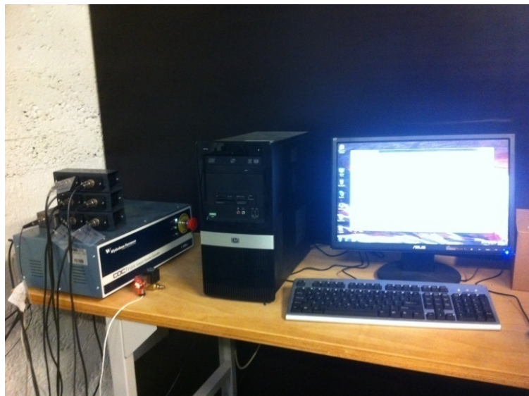
Figure II.22. Compact dynamic controller, data acquisition card and controlling computer
