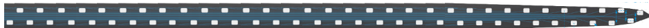
Figure 1.1: The laminar electrode used during ER experiment at UNIC lab. It has 64 recording points staggered along a silicon array. This Figure is extracted from technical documentation of Neuronexus and edited by Yannick Passarelli.
