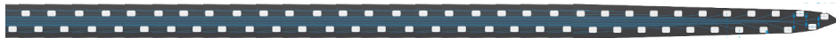
Figure 1.1: The laminar electrode used during ER experiment at UNIC lab. It has 64 recording points staggered along a silicon array. This Figure is extracted from technical documentation of Neuronexus and edited by Yannick Passarelli.
