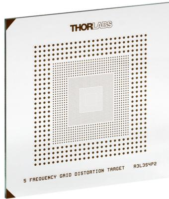
Figure 3.15 – ThorLabs grid distortion target. 3in x 3in, 125 to 2000  $\mu\text{m}$  grid spacings, soda lime glass.
