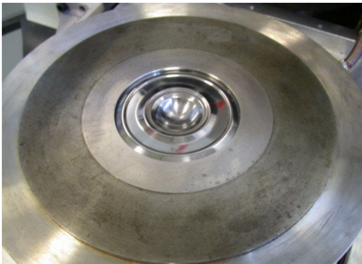
Fig. 3.3. The lower die of the CONAC 40 press. The cone shaped hole is clearly visible in the centre of the die.
