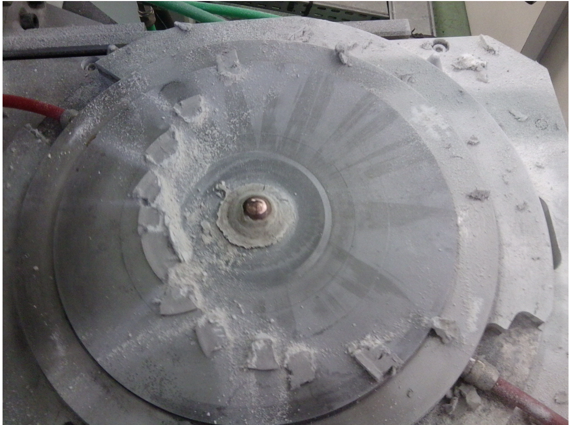
Fig. 3.11. The explosion of a CONAC pressure cell. Notice the radial trajectories caused by the flying debris.
