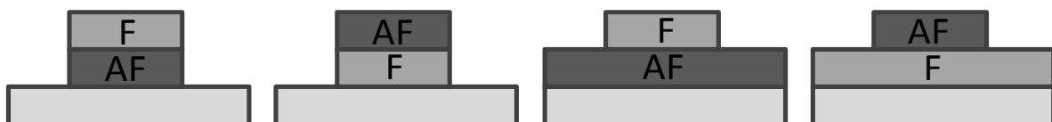
Fig. 1.16 – Sketches of possible nanopatterned configurations for exchange biased dots.
