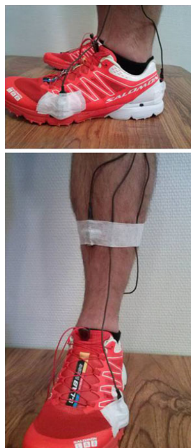
Fig. 1 Placement of the three accelerometers on the left leg of the subject: on the tibia (at the distal third from medial malleolus to great trochanter on the bone's anteromedial aspect), on the external side of the shoe at the fifth metatarsal's head (above the midsole) and on the back of the shoe at the heel (above the midsole). Accelerometers were firmly taped with strapping and Dual Lock™
