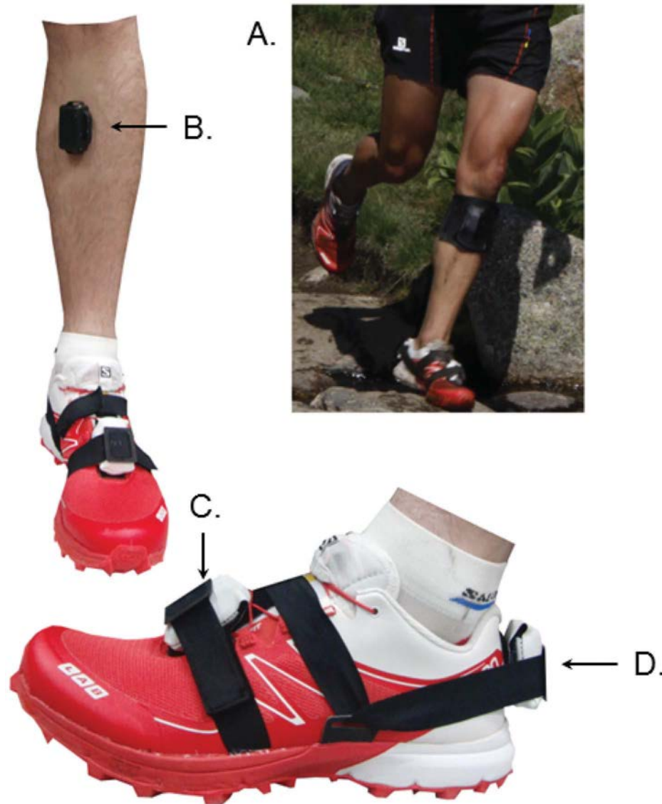
Figure 1. Placement of the three accelerometers. Panel A represents the accelerometers' placement and attachment onto the subject during the race. Panel B illustrates the placement of the tibial accelerometer without the attachment system, for more clarity. Panels C and D show more precisely the placement and attachment of the metatarsal and heel accelerometers, respectively.
