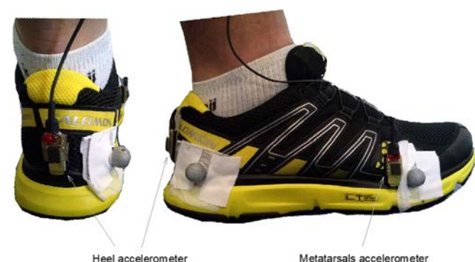
Fig. 2. Placement of the two accelerometers and two retroreflective markers on the subject's right shoe. The heel accelerometer is placed on the back of the shoe at the heel (above the midsole). The rearfoot marker is placed on the external side of the shoe at the heel (above the midsole). Metatarsal accelerometer and forefoot marker are placed on the external side of the shoe at the head of the fifth metatarsal (above the midsole). All accelerometers and markers are firmly taped with strapping and Dual Lock™. For more clarity, straps are not put onto the accelerometers in this picture.
