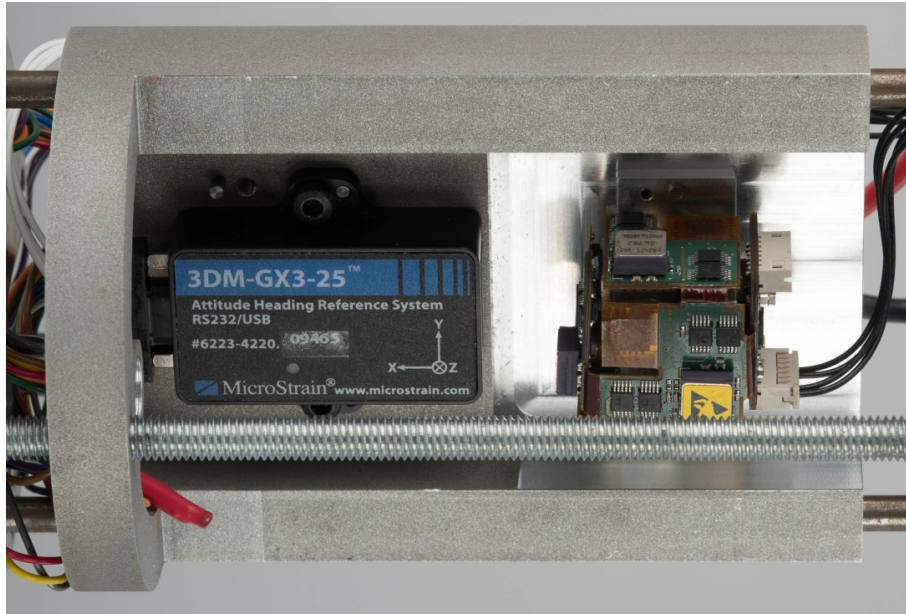
FIGURE 1.12: ACHILES Inertial sensors. Left: Microstrain 3DM-GX3 IMU, Right: MBDA Germany Mini-IMU (not used in this study).
