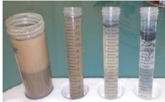
Figure 6.7: SCGc extraction from soil. From left to right: soil:H 2 O (1/1) mix; sampling supernatant; repeated washing. The floating biochar is extracted and stored for analysis.
