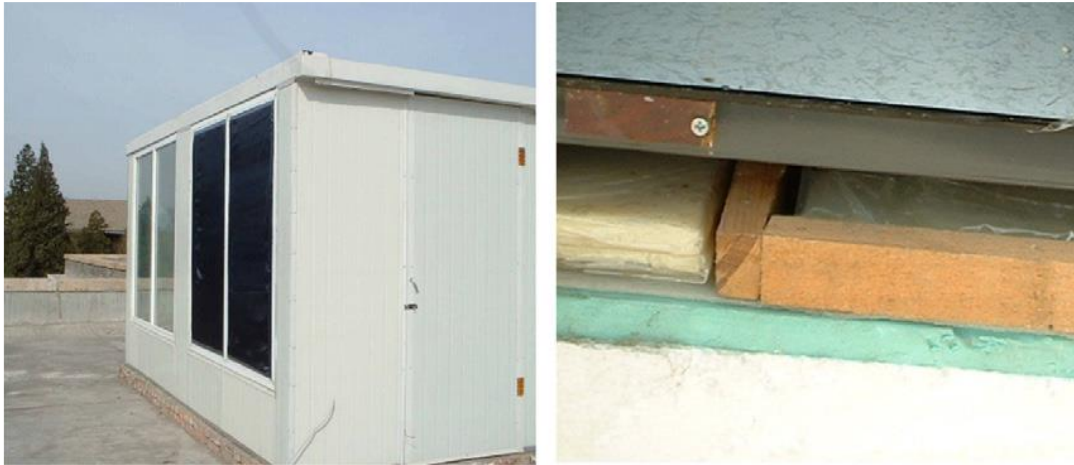
Figure 2.25: Lin et al. experimental house and enhanced floor heating system.
