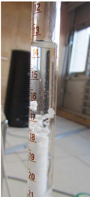
Figure 3.15: PCM during liquefaction
