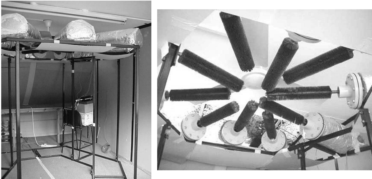
Figure 2.27: Turnpenny et al. LHS unit, overall view (left) and heat exchange pipes (right)
