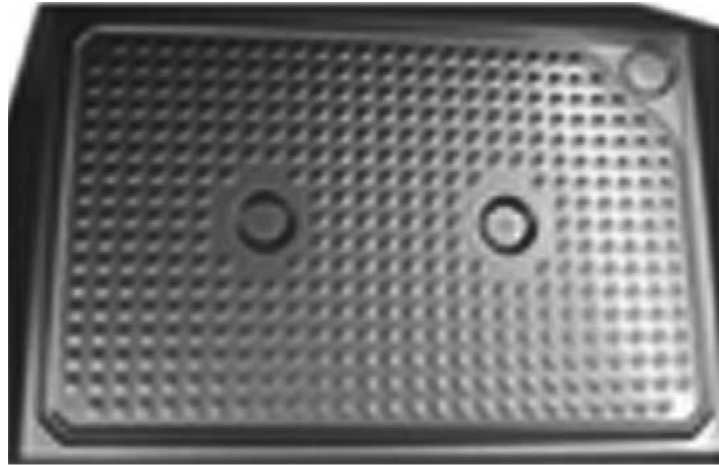
Figure 2.20: Lazaro et. al LHS second encapsulation method (aluminum panels)
