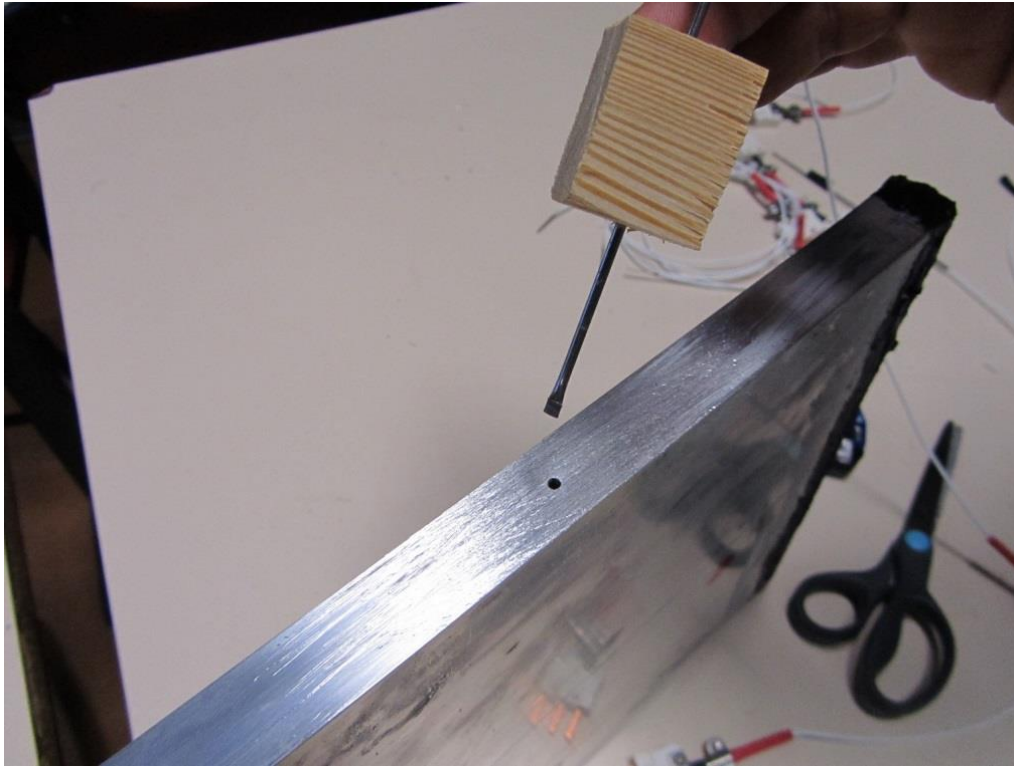
Figure 3.11: Insertion of temperature sensors inside the PCM
