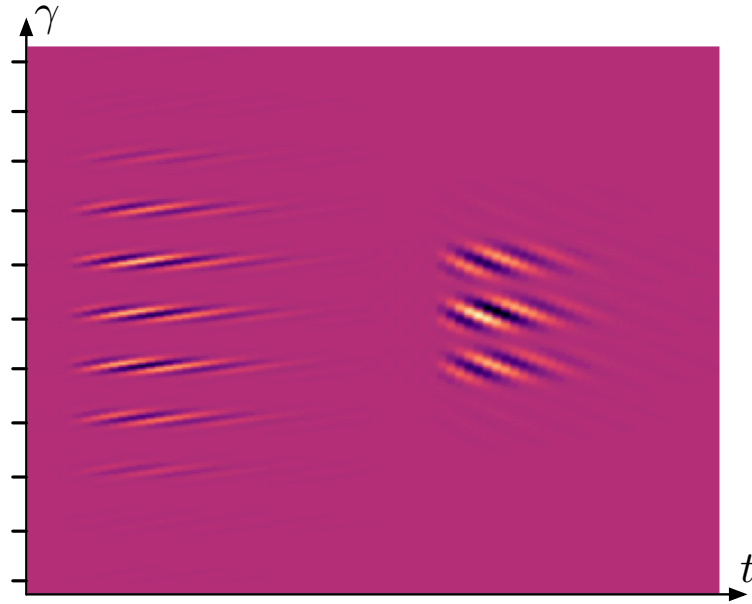
Figure 4.11: Spiral wavelets in the time-frequency domain. Brighter colors denote greater algebraic values of the real part. The background color corresponds to a null real part. Ticks on the vertical axis denote octave intervals.
