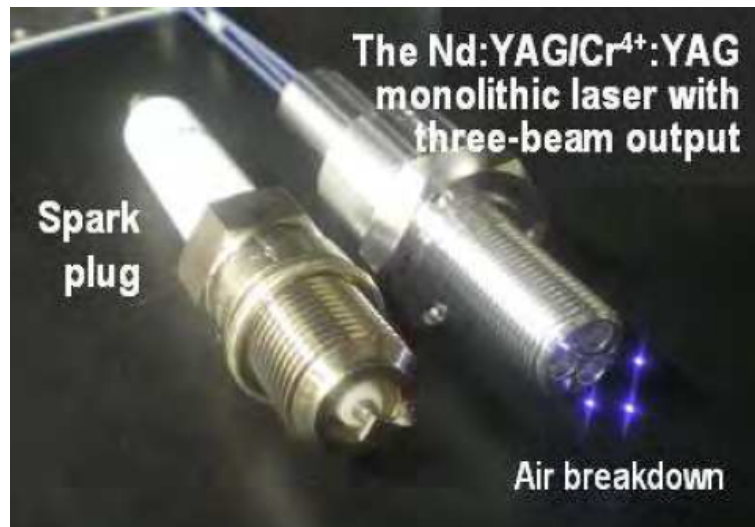
FIGURE 1.34 – Prototype d'allumeur laser multi-points [98]
