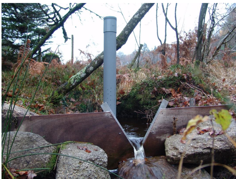
Figure 4-2. V-notch weir and float-operated stage logger in its stilling well at Rocher.
