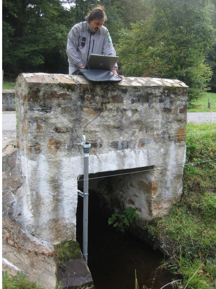
Figure 4-3. Gauging station at the catchment outlet, with the pressure logger in its stilling well..
