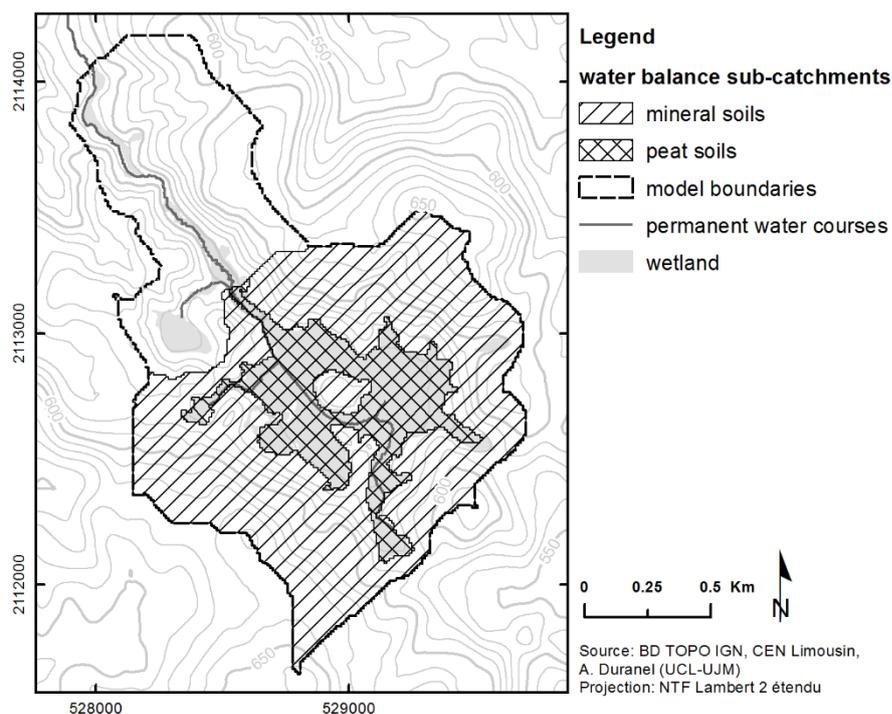
Figure 7-7. Water balance sub-catchments.
