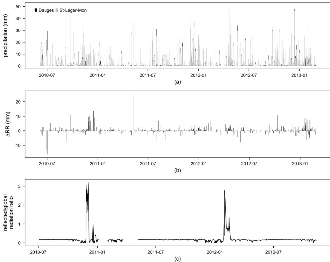
Figure E-32. Impact of snow fall events on the difference between precipitation records at the Dauges site and at the Saint-Léger-la-Montagne station.
