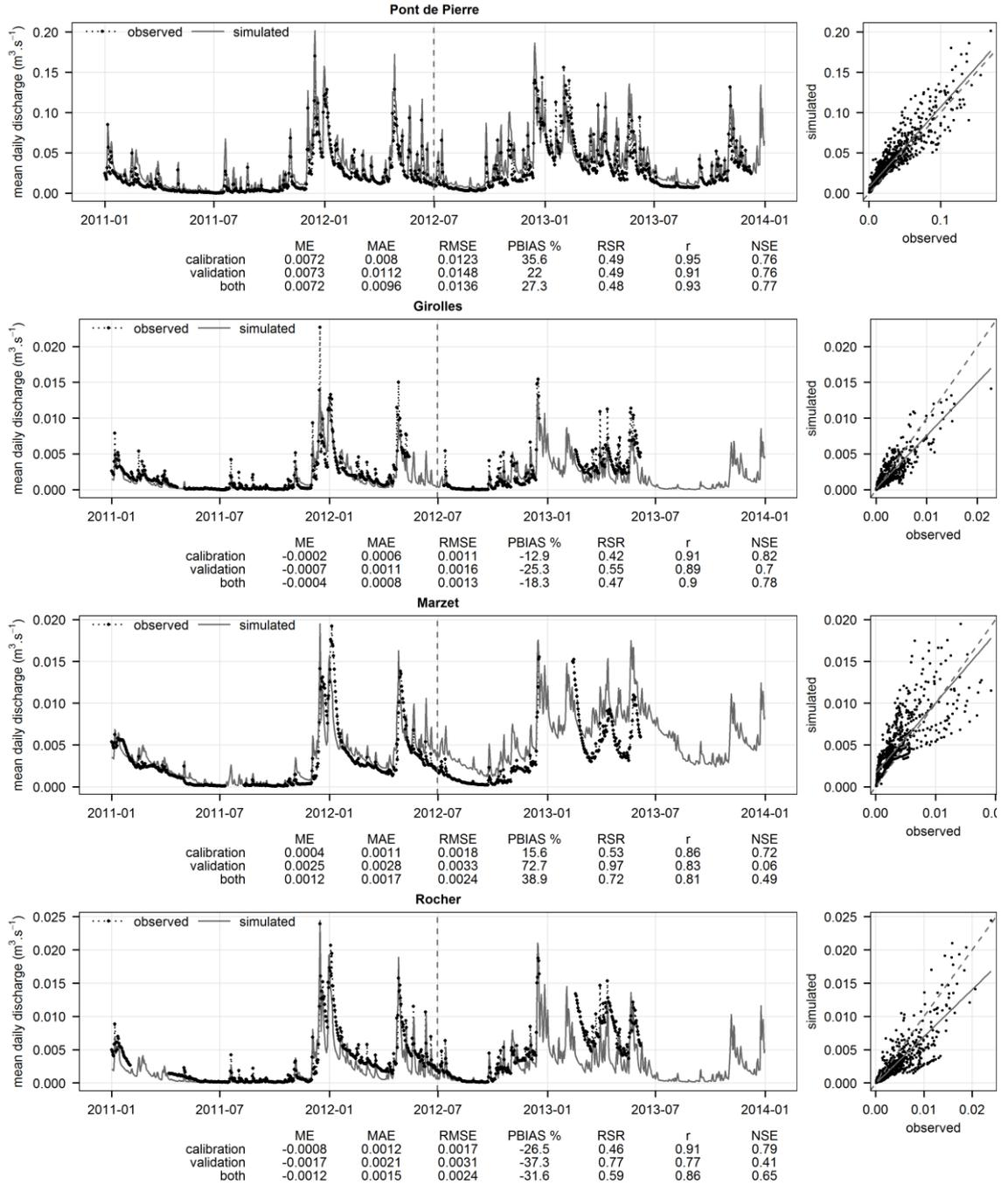
Figure 6-3. Observed and simulated stream discharge (calibrated model).
