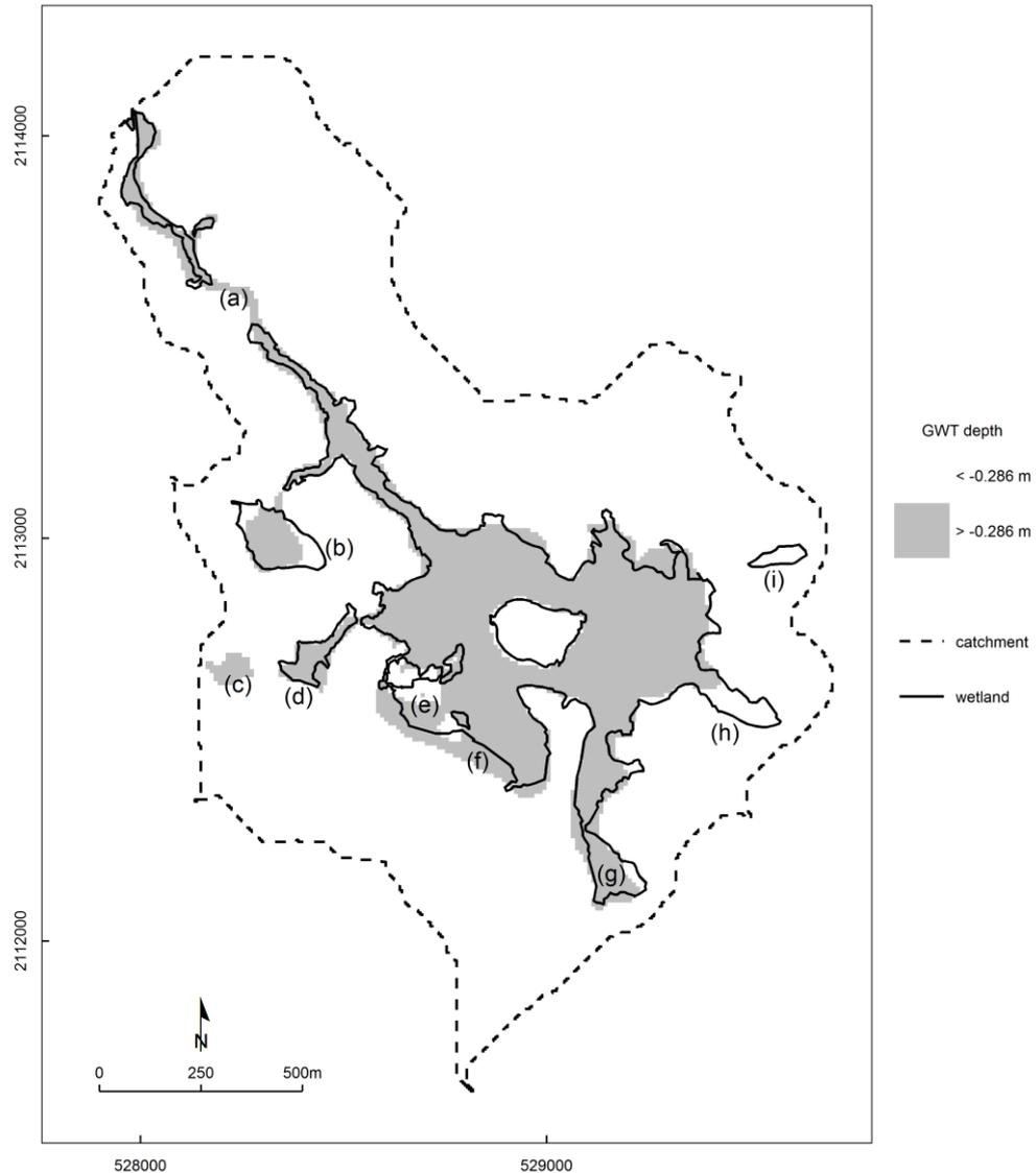
Figure 6-6. Spatial distribution of shallow groundwater tables (2011-2013 mean higher than -0.286m below ground level) and of wetland vegetation.
