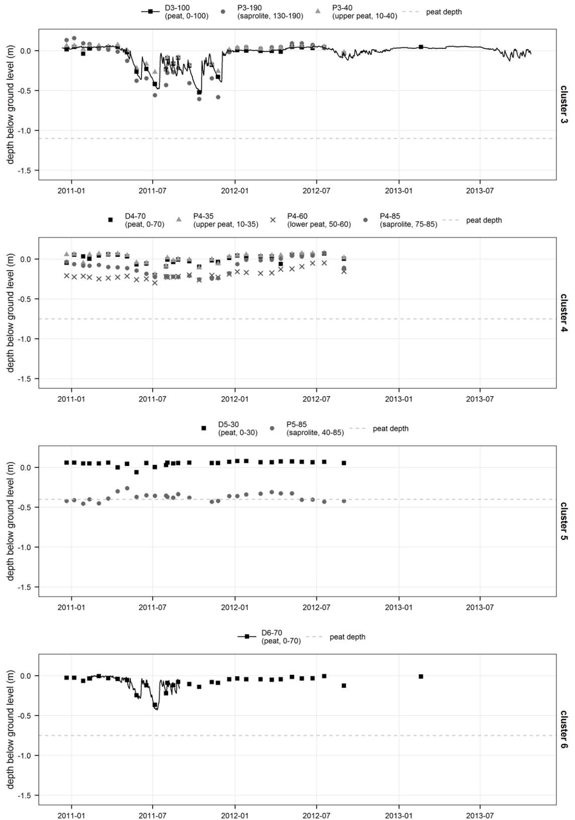
Figure 4-23. Time series of piezometric heads in clusters 3-6.
