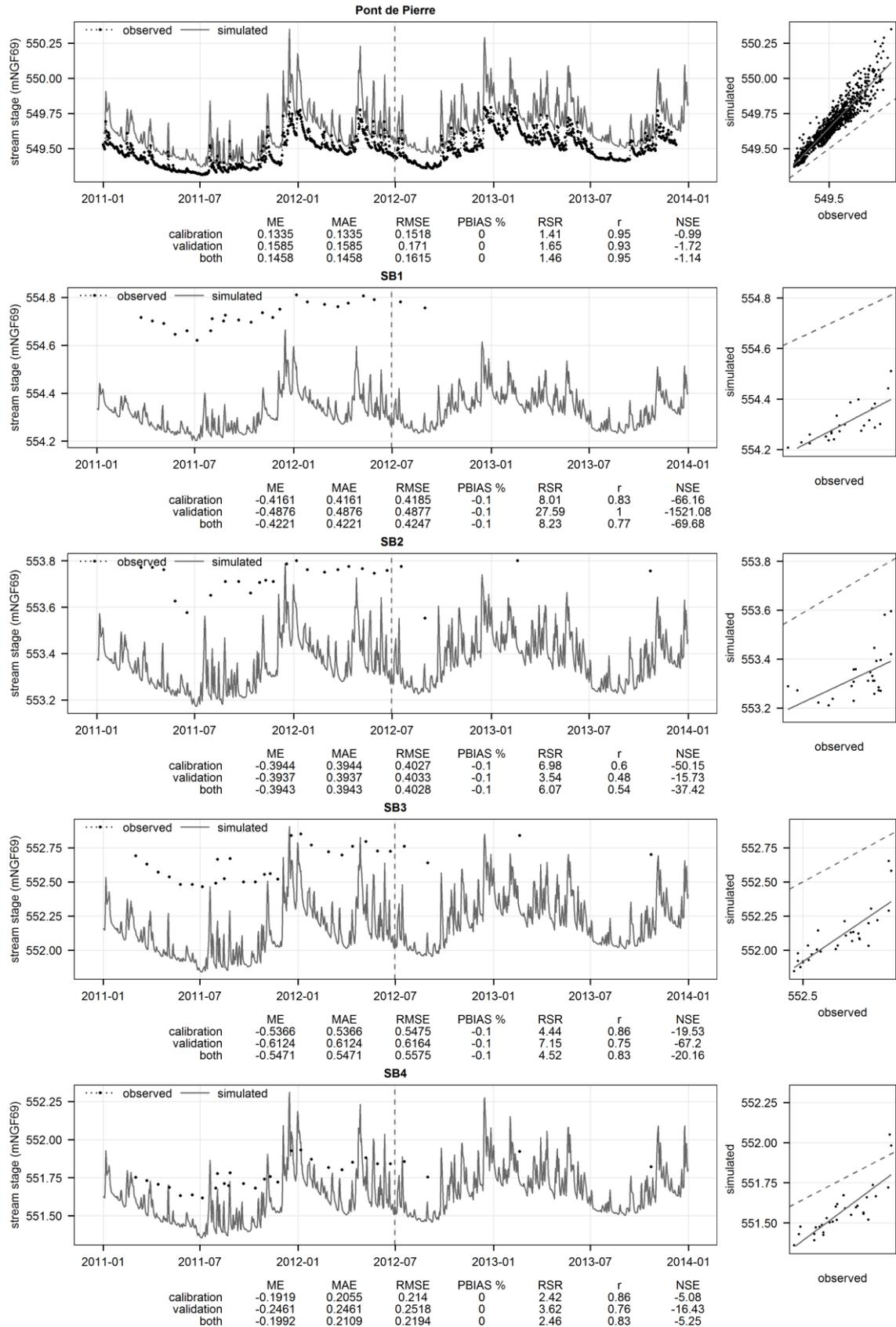
Figure 6-4. Observed and simulated stream stage (calibrated model).
