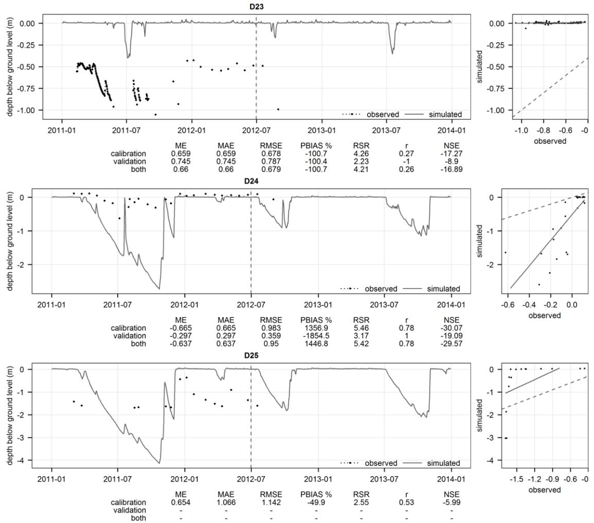
Figure 6-5 (continued). Model performance with regard to groundwater table depth (calibrated model).
