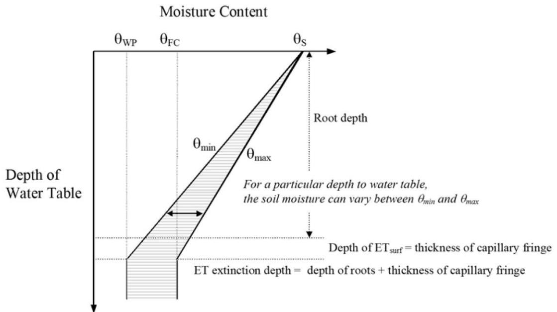
Figure 5-3. Allowable water content in the upper layer of the two-layer unsaturated zone model, as a function of water table depth (from Anonymous 2009c).
