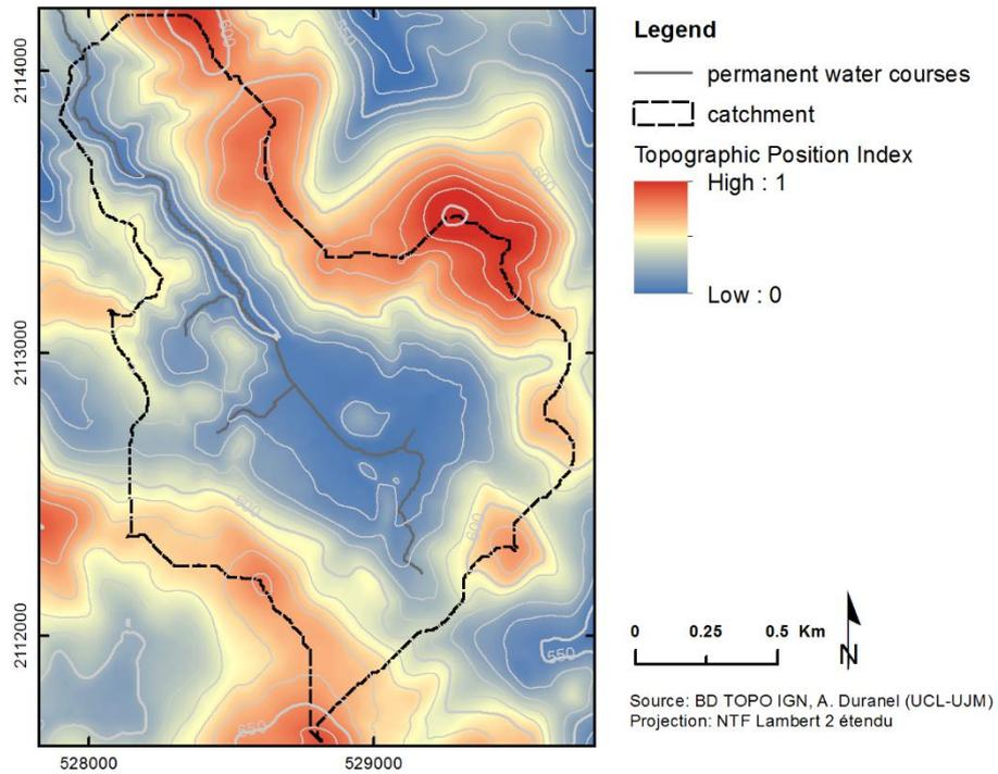
Figure 6-7. Topographic position index (scaled to 0-1 range).
