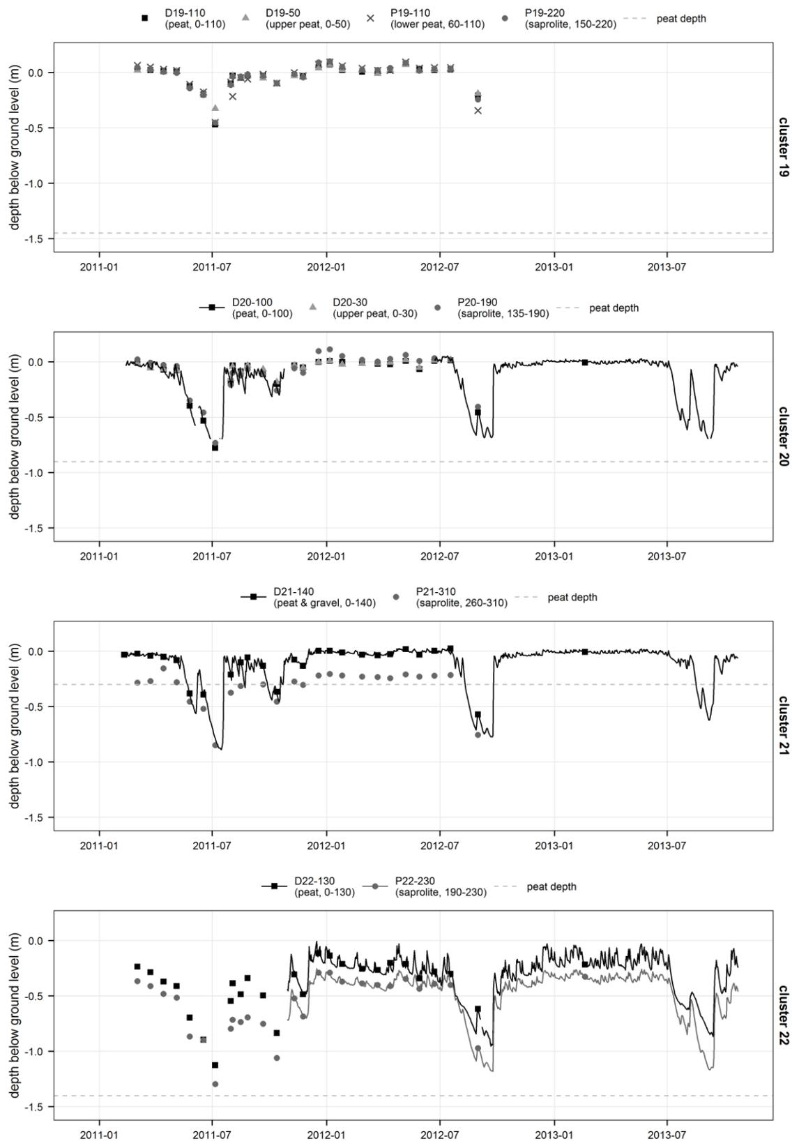
Figure 4-27. Time series of piezometric heads in clusters 19-22.
