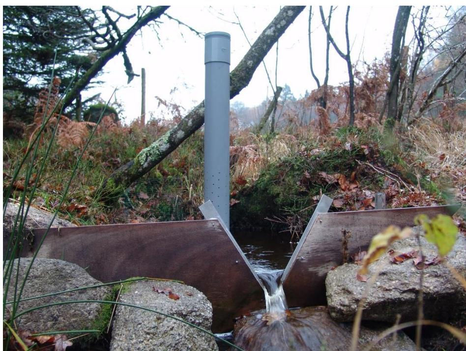
*Figure 4-2. V-notch weir and float-operated stage logger in its stilling well at Rocher.*
