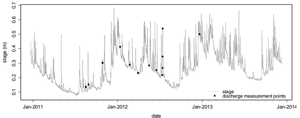
Figure 4-9. Stream stage at the Pont-de-Pierre gauging station.
