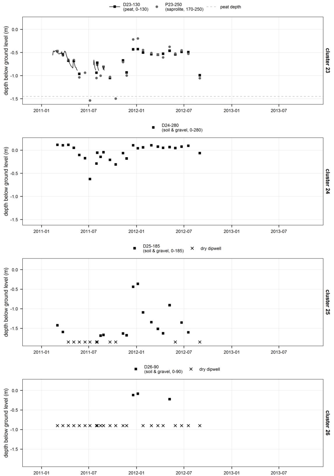
Figure 4-28. Time series of piezometric heads in clusters 23-26.
