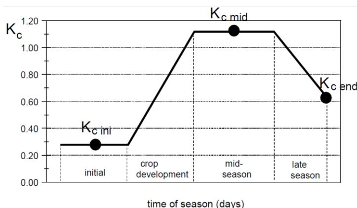
Figure 5-14. Idealised crop coefficient curve (Allen *et al.* 1998).
