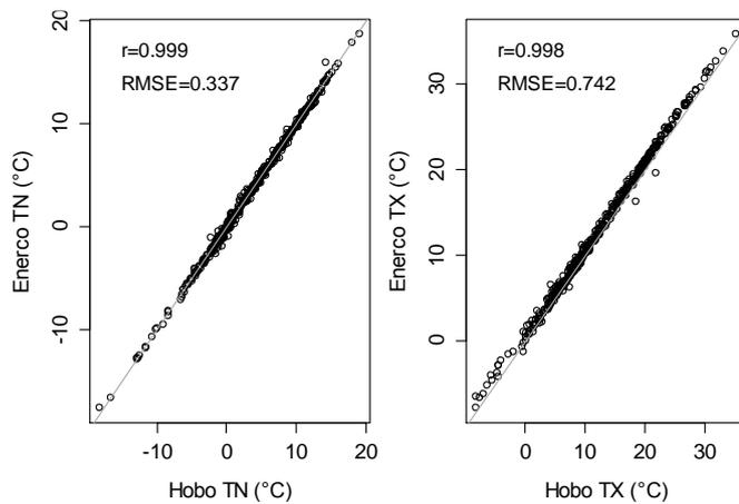
Figure E-8. Scatterplots of temperature extremes recorded by the Enerco and Hobo loggers at the Dauges site.
