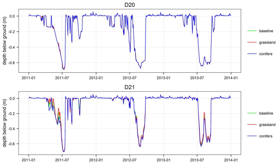
Figure 8-8 (continued). Impacts of catchment landuse on simulated groundwater table depth in a selection of dipwells within the mire (01/01/2011-31/12/2013).
