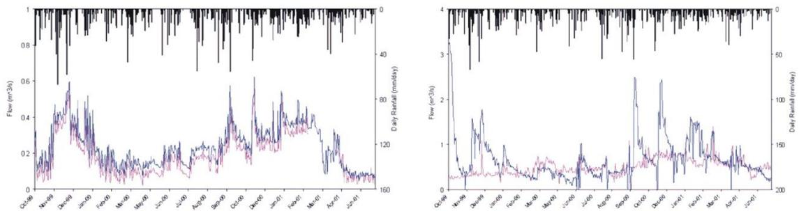
Figure 5-8. Observed and simulated discharge in the Paya Indah wetlands (Rahim et al. 2012).
