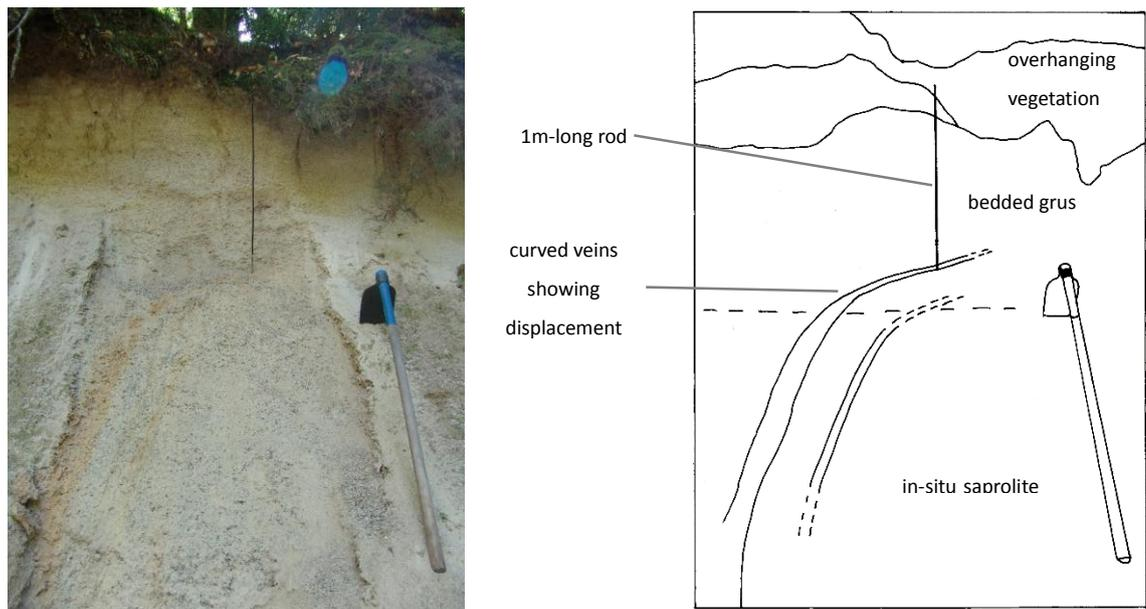
Figure 3-12. Section 2 - close-up view of the downslope side of the quarry.
