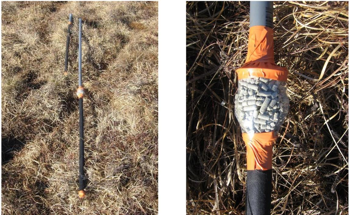
*Figure 4-17. Dipwell and piezometer before installation in the ground.*
