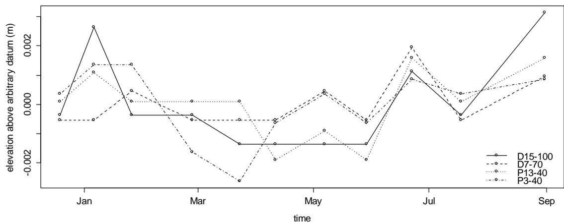
Figure 4-18. Movements of selected shallow piezometers relative to an arbitrary datum.
