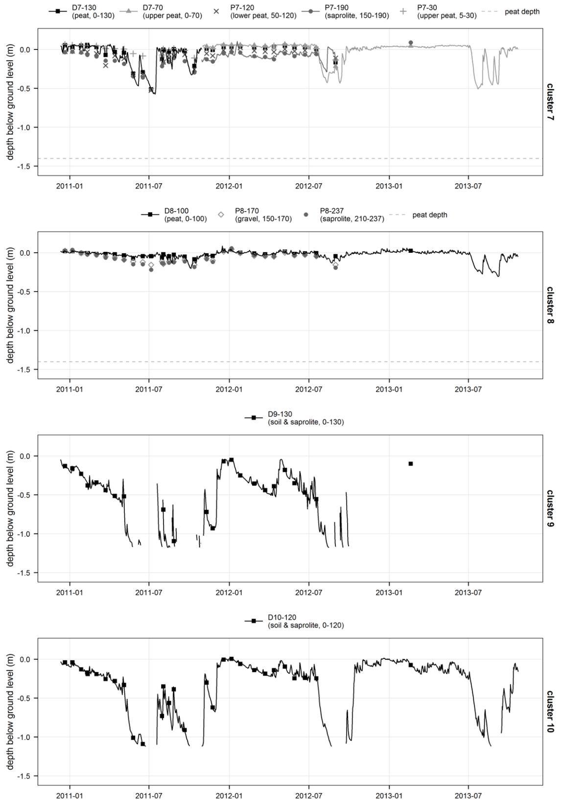
Figure 4-24. Time series of piezometric heads in clusters 7-10.
