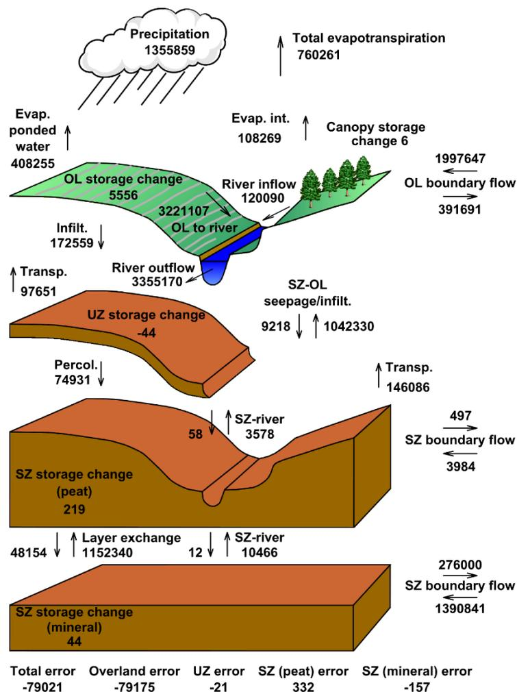
Figure 7-8. Simulated water balance of the mire area upstream of Pont-de-Pierre from 01/01/2011 to 31/12/2013 (m<sup>3</sup>).
