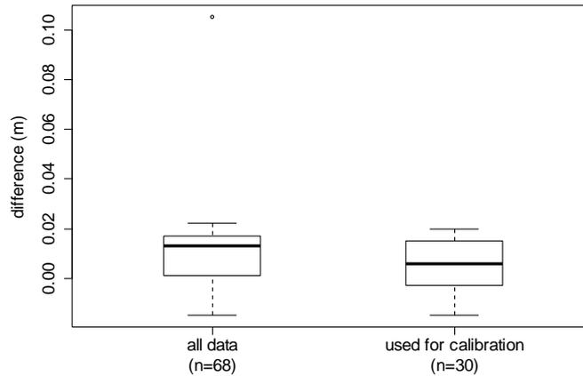
*Figure 4-19. Boxplots of water table height manual reading errors, as estimated by the difference between readings made with the manual dipper and with a tape measure. The right boxplot shows the estimated errors of manual readings used to calibrate logger data.*
