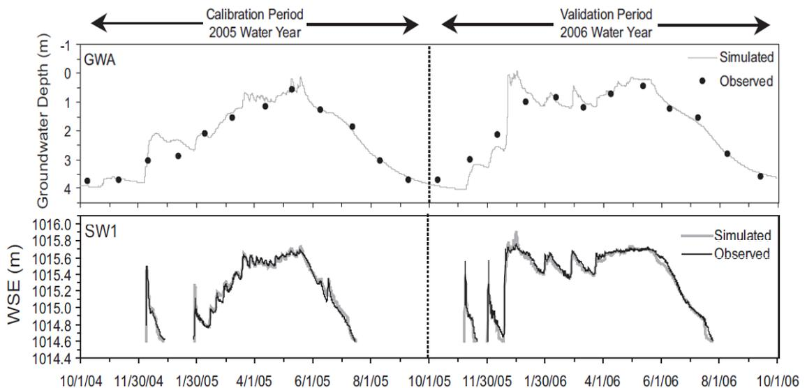
Figure 5-7. Observed and simulated groundwater table depth (top) and stream stage (bottom) in Bear Creek Meadow (modified from Hammersmark *et al.* 2008).
