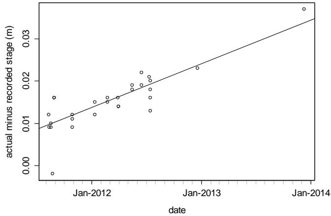
Figure 4-8. Logger drift at the Pont-de-Pierre gauging station.
