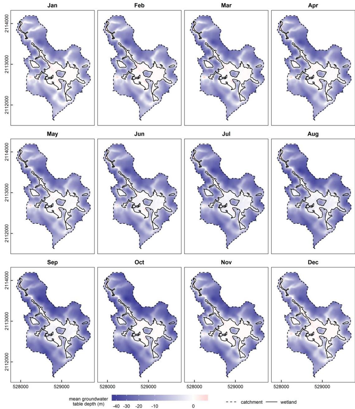
Figure 7-4. Simulated monthly mean groundwater table depth (01/01/2011-31/12/2013).
