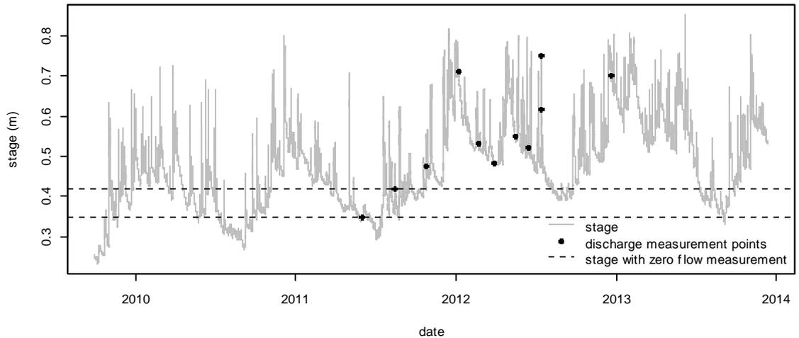
Figure 4-5. Stream stage at the D78 gauging station.
