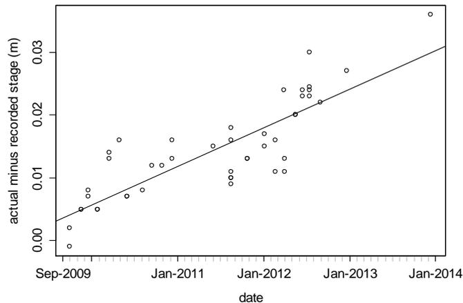
Figure 4-4. Logger drift at the D78 gauging station.
