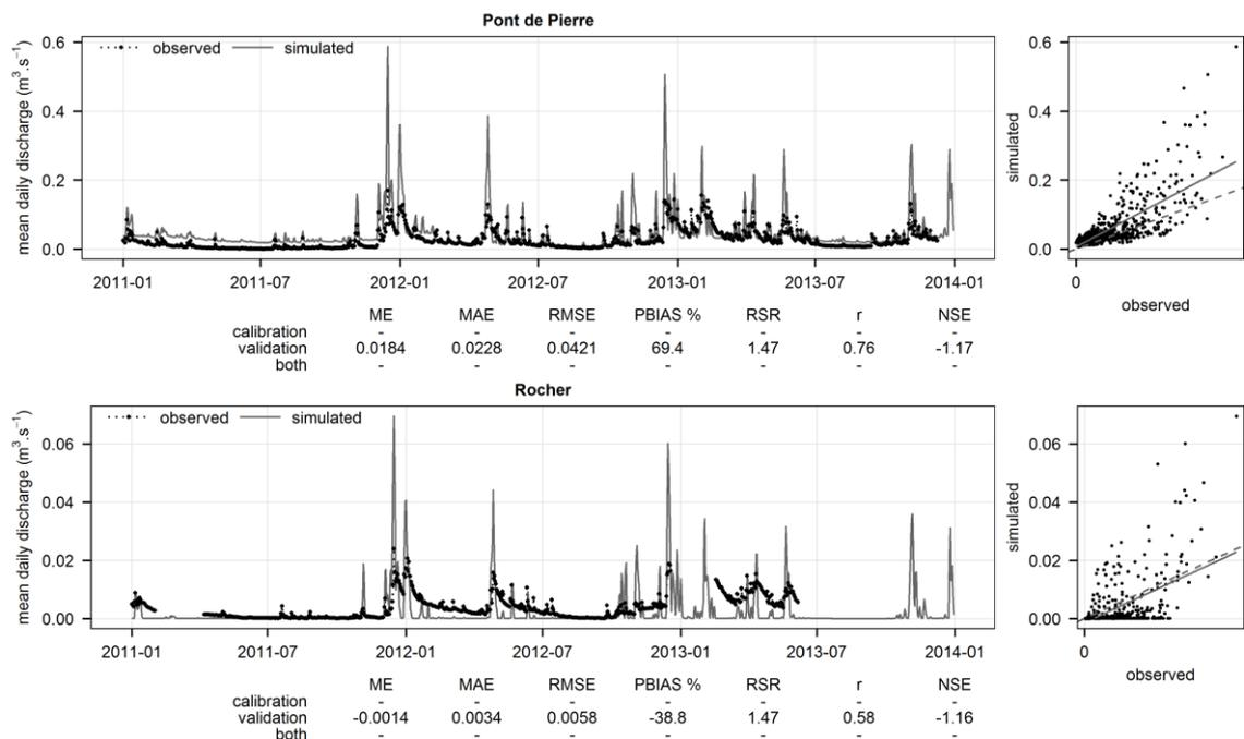
Figure 6-1. Observed and simulated stream discharge (uncalibrated model).
