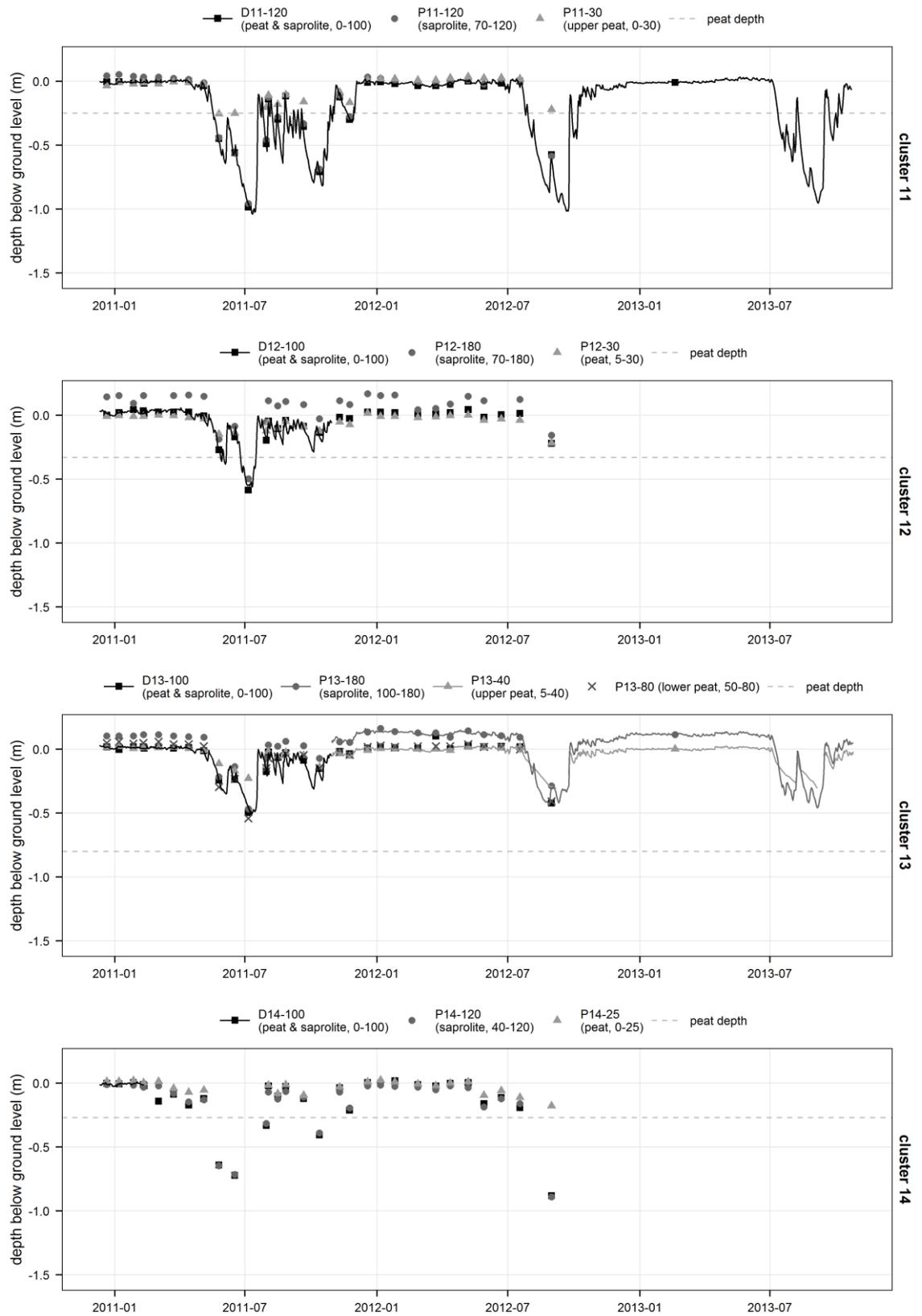
Figure 4-25. Time series of piezometric heads in clusters 11-14.
