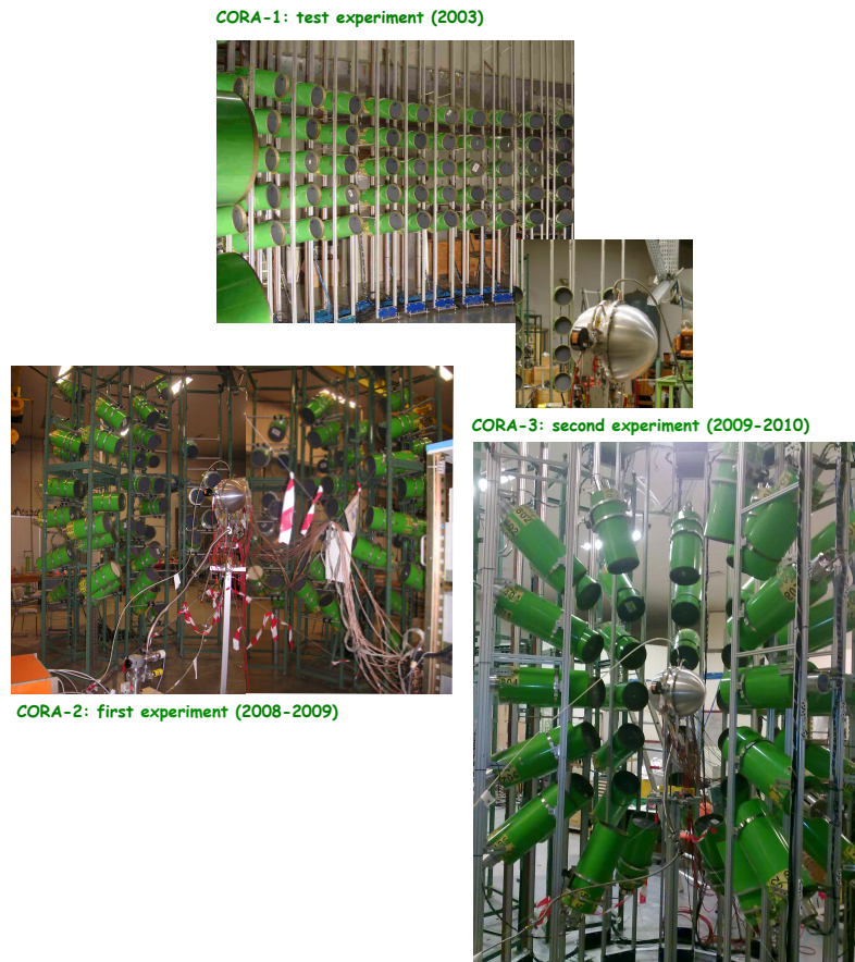
Figure 1.15: The three DEMON configurations are shown. In CORA-1 a wall configuration is used. This experiment represents a preliminary test to demonstrate the existence of the CMs anisotropy; CORA-2: two curved wall arrangements of the detector. The detectors appear shifted respect to each other. This configuration was optimized to avoid the cross talk effect, but the shifted arrangement could have induced neutron scattering on the mechanical supports. To avoid scattering for CORA-3 experiment a near-spherical configuration was preferred.
