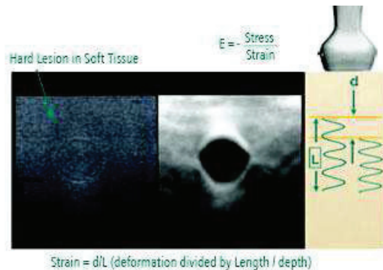
Figure 1.2 Comparison between sonograms (left) and a strain map (right) in a tissue mimicking phantom. Source: medical.siemens.com
