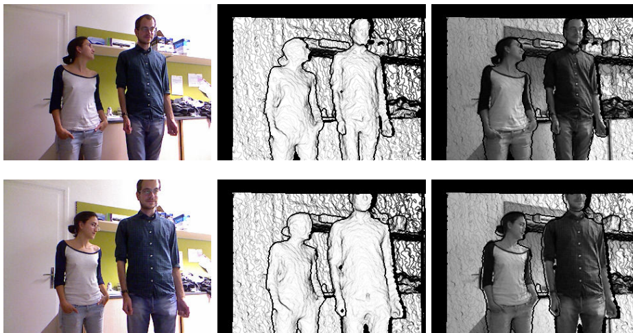
Fig. 6.9: Large Z -motion experiment proposed by Hornacek et al. (2014) . From left to right: (a) color image, (b) 3D surface and (c) RGBD image. First and second images are presented in the top and bottom rows, respectively. The experiment estimates the motion in both directions.
