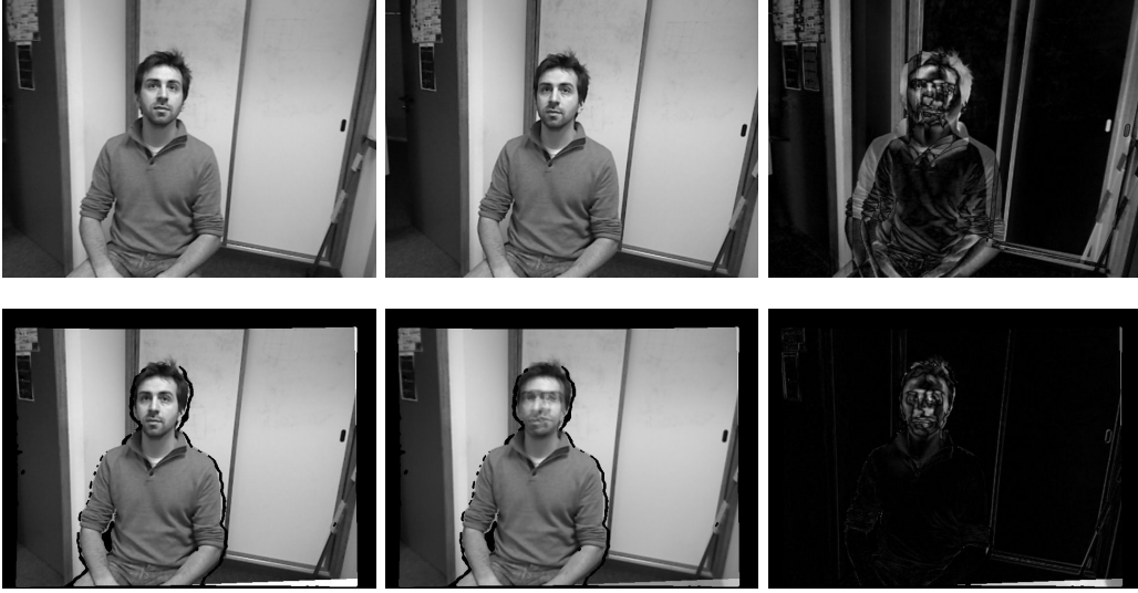
Fig. 5.7: Rigid motion compensation. From left to right, top to bottom: (a) first image, (b) second image, (c) difference between input images, (d) second image warped to compensate rigid motion, (e) image blended using first image and the compensated, and (f) difference between first image and the compensated. Once the rigid motion has been compensated the motion estimation becomes the computation of the nonrigid residual of the motion.
