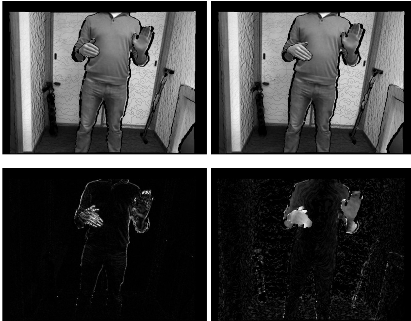
Fig. 5.1: RGBD changes using a fixed camera. Form left to right, top to bottom: (a) first image, (b) second image, and absolute difference in (c) intensity and (d) depth. Moving surfaces produce changes in intensity and depth, while static scene points remain unchanged, except by the noise.
