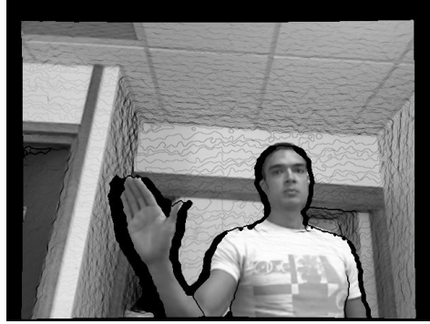
Fig. 2.2: The RGBD image is displayed by showing the gray valued of every pixel having a valid depth measure. We also incorporate information about 3D structure as contour lines, which are defined as a function of the point-wise changes in depth data.
