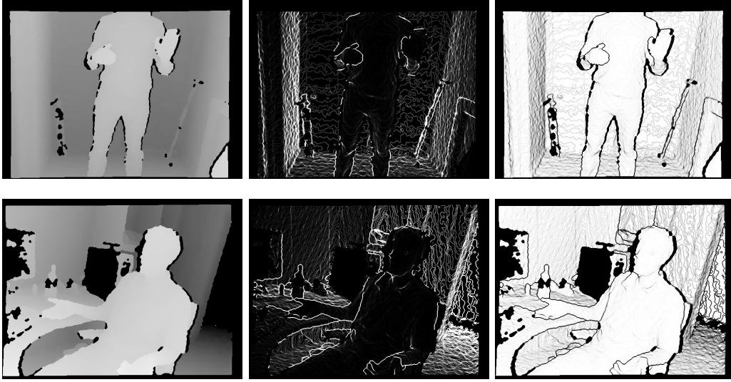
Fig. 5.5: Depth-based discontinuities preserving. From left to right: (a) depth image, Z(x) , (b) magnitude of the gradient, |\nabla Z(x)| , and (c) depth-based weighting function, c(x) .
