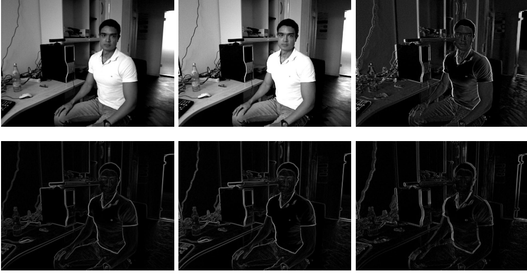
Fig. 5.3: Brightness constancy violation. From left to right, top to bottom: (a) first image, (b) second image, (c) image difference, (d) first and (e) second images of the magnitude of the gradient, and (f) their difference. While the camera is moving, there exists an automatic white balance that modifies the gray value image, as can be noted in the image difference (c), changes that are not related to the motion. On the other hand, the magnitude of the gradient is too little affected since it measures the image structure, or texture, regardless uniform changes in luminance.
