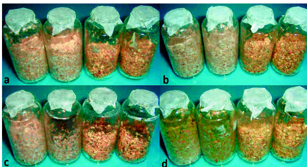
Figure 3.3. Pictures of SSF for enzymatic cocktail production with the two biomasses (two left glass flasks: wheat bran; two right flasks: corn cobs). a: A. terreus 826. b: A. terreus 62071. c: A. tubingensis . d: A. oryzae .
