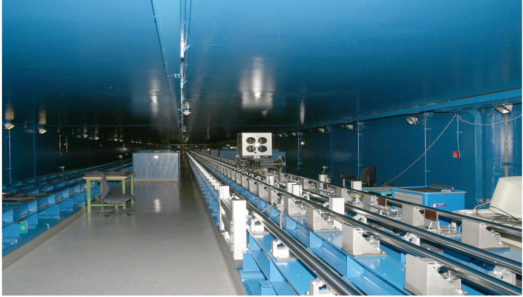
FIGURE 3.6: VLTI delay line. Credit: ESO
