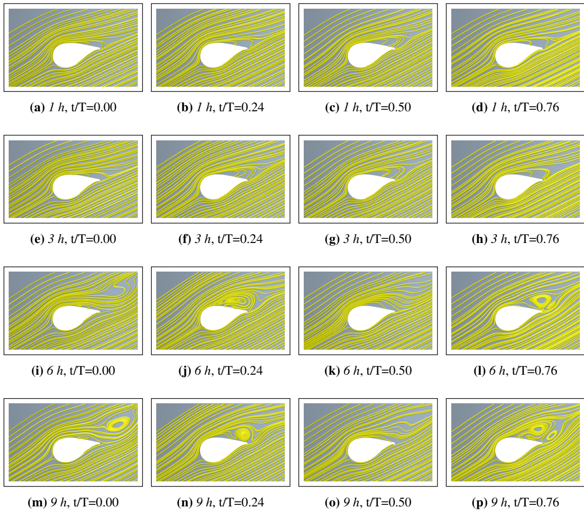
Figure 6.7: Relative velocity streamlines around the observed blade for a r/R=0.22 cross-section and different time reconstructed solutions
