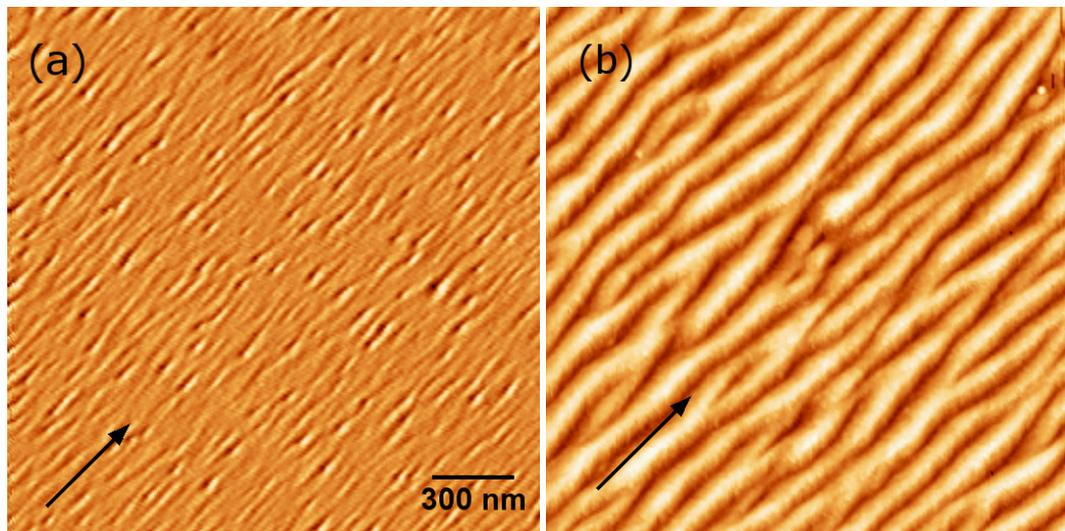
**Figure 4.10:** 5 nm  $\text{Si}_{0.7}\text{Ge}_{0.3}$  deposited on  $10^\circ$  substrate at  $500^\circ\text{C}$ , (left) As-grown sample and (right) after post-growth 18-hour annealing at  $500^\circ\text{C}$ , [110] direction is indicated by black arrow and the images size is  $2 \times 2 \mu\text{m}^2$
