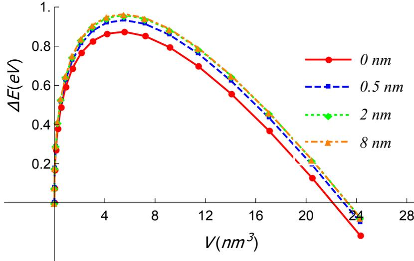
**Figure 3.10:** The energy variation  $\Delta E^{total}$  as a function of  $V$  of PB while varying the distance  $d$  from PA, marked as different colors, red, green, blue and yellow respectively for  $d = 0$  nm,  $d = 0.5$  nm,  $d = 2$  nm and  $d = 8$  nm.
