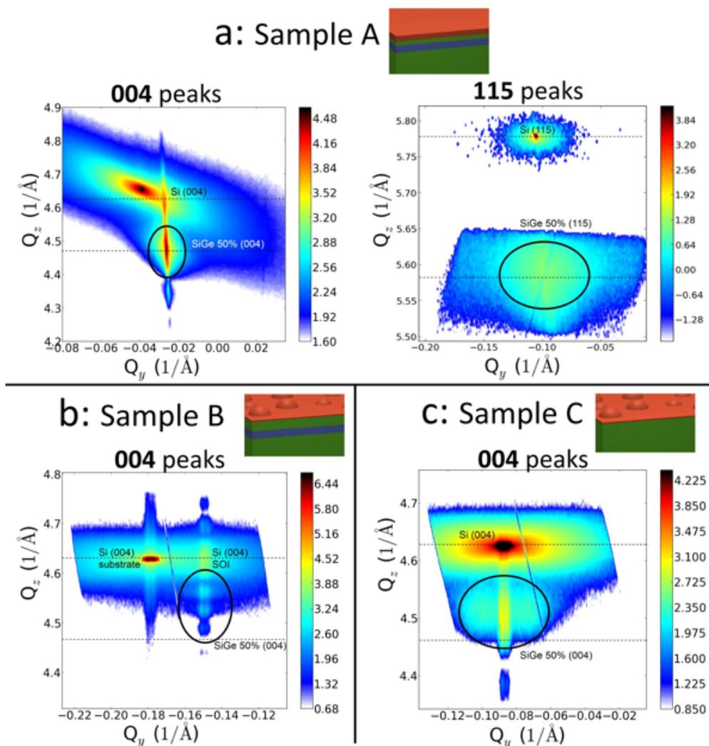
**Figure 5.7:** (a) Reciprocal space maps (RSMs) around 004 (left panel) and 115 (right panel) Si and SiGe Bragg peaks of sample A. (b and c) RSMs around 004 Si and SiGe Bragg peaks of samples B and C, respectively.
