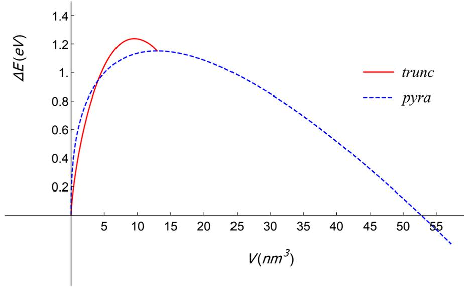
Figure 2.10: The energy barrier variation of truncated pyramid pathway and pyramid pathway.
