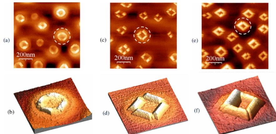
**Figure 1.22:** STM images ( $1 \times 1 \mu\text{m}^2$ ) of the groups of closely spaced SiGe islands grown at 660 °C on a three-layered QD superlattice template with different thickness of deposited Ge:(a) 3.5 MLs, (c) 4 MLs, (e) 5 MLs. Image sides are oriented along the [011] directions. Figures (b), (d), and (f) correspond to three-dimensional representations of the fourfold symmetric QDMs, marked by dash circles in (a), (c), and (e), respectively[35].
