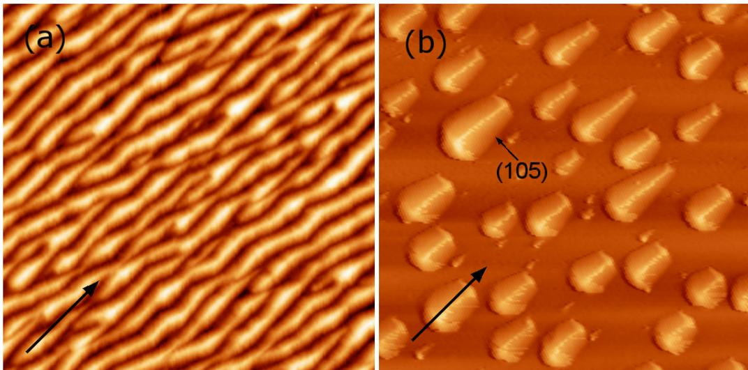
**Figure 4.11:** 5 nm  $\text{Si}_{0.7}\text{Ge}_{0.3}$  deposited on  $10^\circ$  substrate at  $500^\circ\text{C}$ , (a) after post-growth 72-hour annealing at  $500^\circ\text{C}$ . and (b) after post-growth 72-hour annealing at  $575^\circ\text{C}$ ,  $[110]$  direction is indicated by black arrow.
