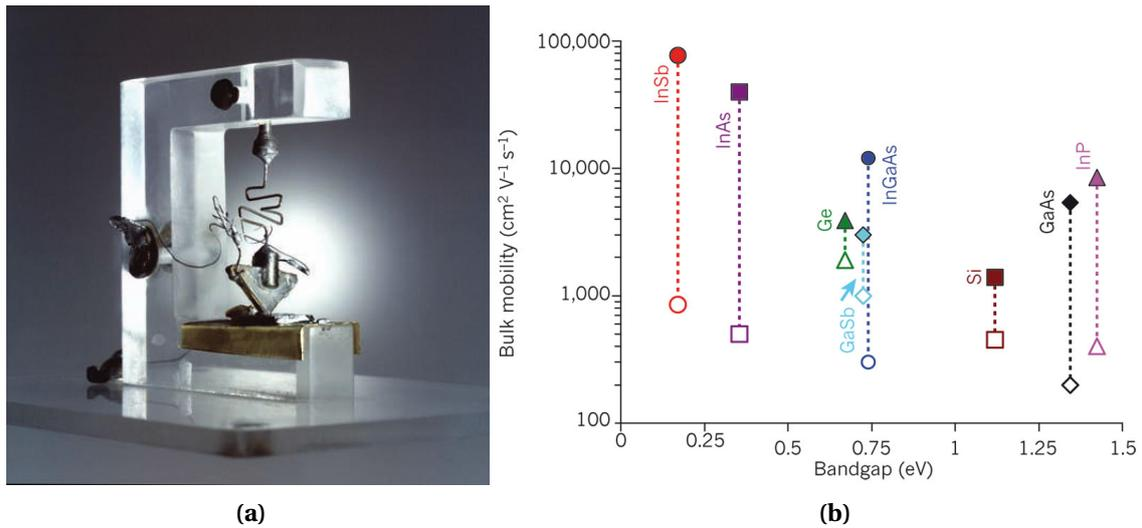
**Figure 1.2:** (a) The first transistor in the world made of Ge. (b) The mobility landscape of semiconductors. The bulk mobility is plotted against the bandgap for silicon, germanium and a variety of group III-V materials. Filled symbols indicate electrons, and open symbols indicate holes. Germanium offers the highest hole mobility of any known semiconductor material [7],
