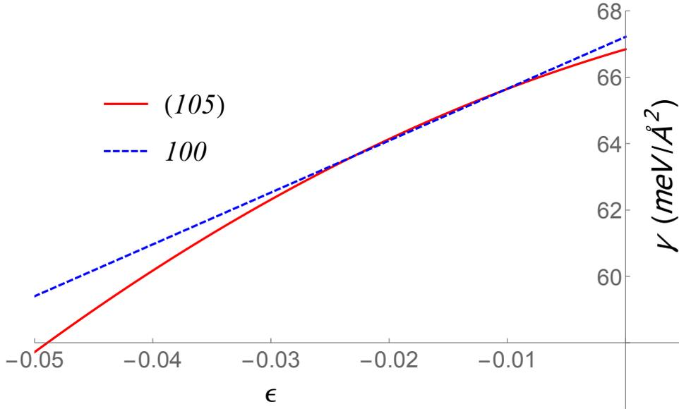
**Figure 3.5:** The strain-dependent surface energy as a function of  $\epsilon$  for facet(001) and (105) respectively. Note that only reconstruction (2) of facet (001) is considered as the reconstruction transition occurs at low-strain regime, not associated to the strain regime in calculation
