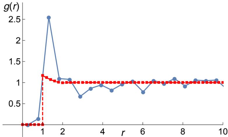
**Figure 3.3:** Distribution function  $g(r)$  (solid blue line) of the islands found experimentally as a function of their distance  $r$  in unit of the mean island diameter  $\sigma$ . The red dashed curve corresponds to the theoretical distribution function of hard-core disks with the same island density (that is  $\phi = 13\%$ ) in the Born-Green-Yvon approximation
