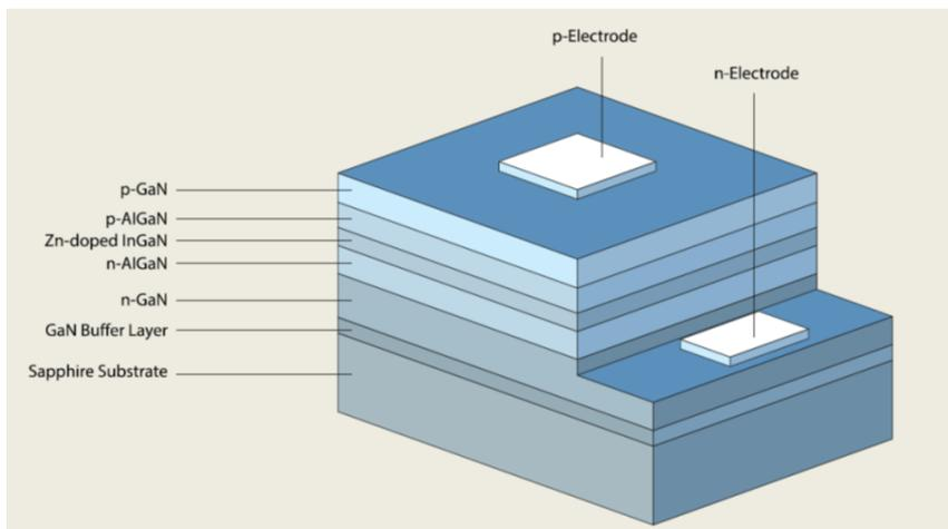
Figure 1.1: Schematic structure of the first blue LED[2]
