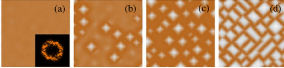
**Figure 1.14:** Numerical simulation of a surface for a 5-nm strained anisotropic film of  $\text{Si}_{0.7}\text{Ge}_{0.3}$  (a) as-grown (Fourier transform in inset), after annealing time of (b) 18h, (c) 54h, and (d) simulation of a 8-nm film after 18h annealing. [The scan area is  $1.2\mu\text{m} \times 1.2\mu\text{m}$ , and the vertical scale is 31 nm.][28]
