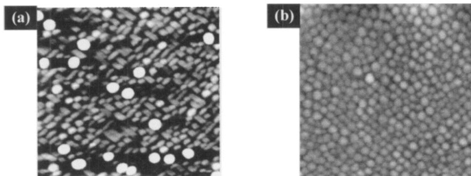
**Figure 1.16:** AFM image of 13ML Ge on (a) Si(001) and (b) with 1/2ML Sb on Si(001) [30]
