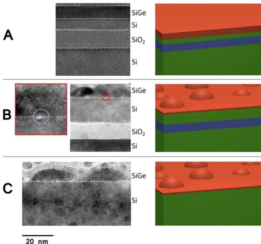
**Figure 5.4:** High-resolution TEM cross-sectional images of the three structures A, B, and C. For each structure, the corresponding schematic representation similar to Figure 1 is presented on the right. For sample B, the inset shows a higher-magnification TEM image to highlight the presence of defects in the crystal.
