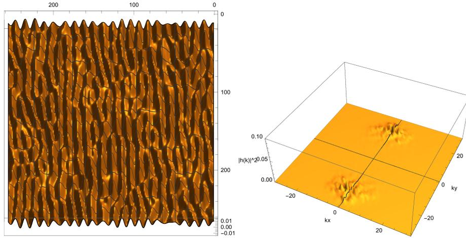
**Figure 4.9:** (left) Anisotropic ATG instability with an asymmetric strain in the  $x$  and  $y$  direction corresponding to the strain asymmetry found experimentally on a vicinal surface corresponding to a time when the peak to peak amplitude of instability is 1 nm; (right) Spectrum of this surface.
