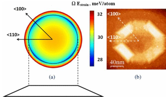
**Figure 1.21:** (a) Simulation by FEM of the surface distribution of strain-dependent chemical potential on the top of a SiGe disklike nanomound covered by a thin Ge wetting layer. The disklike nanomound was represented by a truncated cone with a height to base aspect ratio of 0.05 and a sidewall inclination angle of 14 deg. (b) STM image of spatial ordering of small 3D islands nucleated on the disklike nanomound after deposition of 3.5 MLs of Ge at 600 °C . [35]
