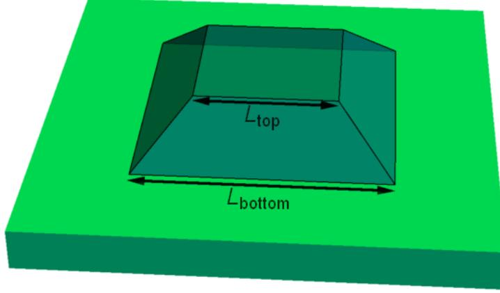
**Figure 2.9:** Schematic figure of a coherent truncated pyramid
