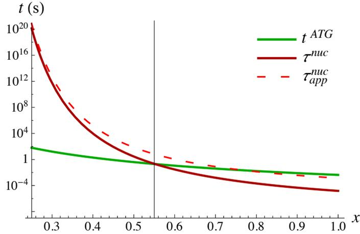
**Figure 2.5:** As a function of composition  $x$ , the nucleation time scale is plotted in red solid curve, characteristic time of ATG instability in green curve and the red dashed curve represents the nucleation time scale which is approximated as in Equation 2.24, and the vertical line marks the crossover composition.
