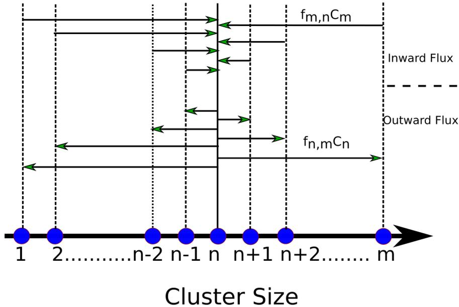
**Figure 2.4:** Schematic presentation of the possible changes in the size of a cluster of  $n$  molecules. The concentration of  $n$ -sized clusters diminishes because of  $n \rightarrow m$  transitions (the arrows leaving size  $n$ ) and increases thanks to  $m \rightarrow n$  transitions (the arrows ending at the size  $n$ ).
