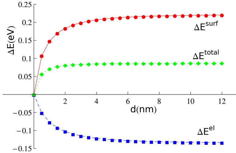
**Figure 3.8:** The energies  $\Delta E^{el}$ ,  $\Delta E^{surf}$  and  $\Delta E^{total}$  as a function of  $d$ , respectively marked in blue, red and green. The points are obtained from numerical calculations and the lines are here for eye-guide.
