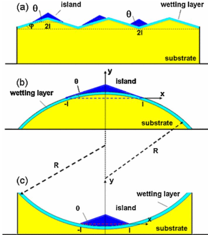
**Figure 1.24:** Schematic illustration of island nucleation on patterned substrates. (a) On a saw-tooth pattern; (b) on the apex of a concave surface; (c) in the valley of a convex surface.[39]
