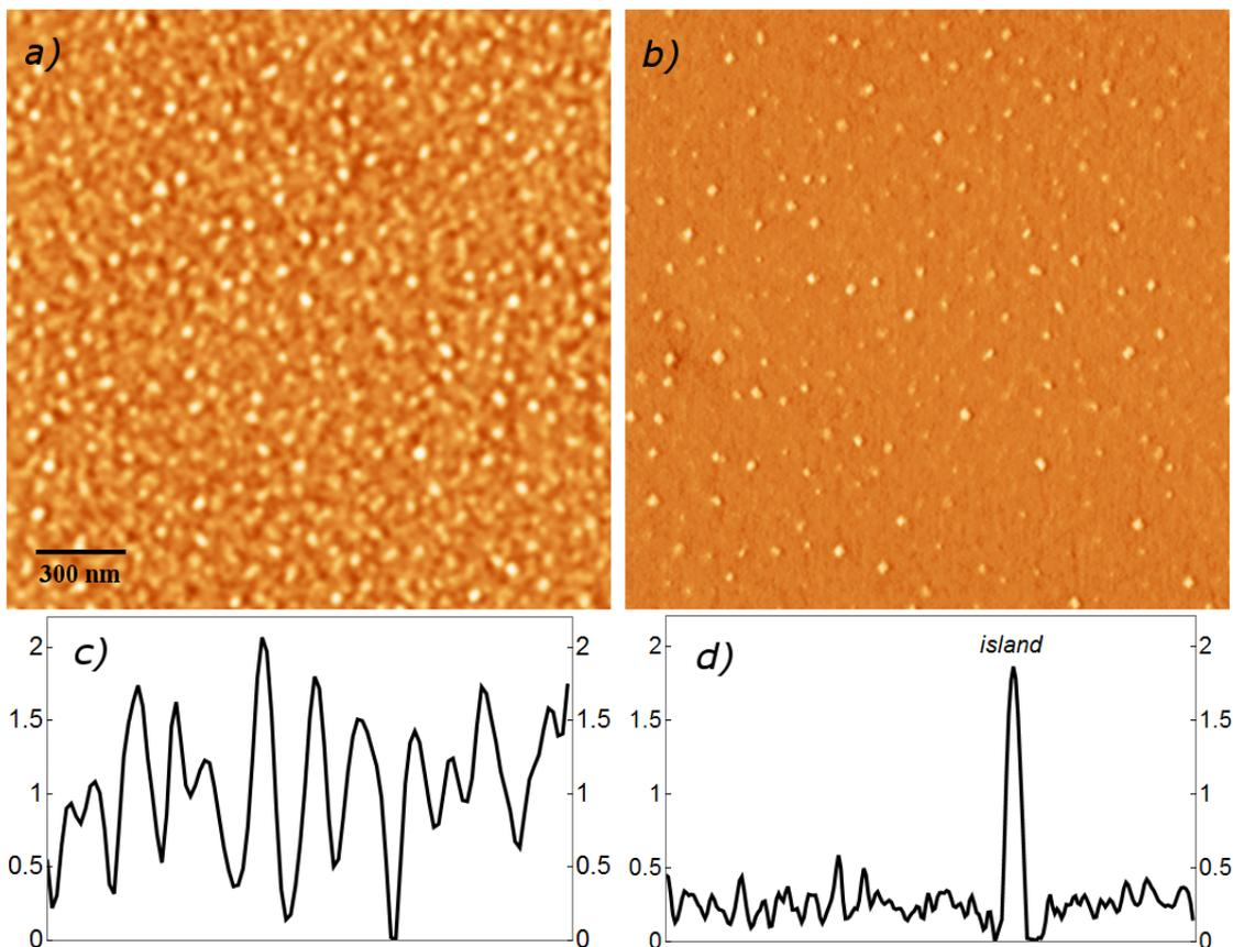
**Figure 2.6:** Experiments to identify cross-over composition  $x_c$ . AFM images of (a) 2 nm Si<sub>0.5</sub>Ge<sub>0.5</sub> and (b) 1.3 nm Si<sub>0.4</sub>Ge<sub>0.6</sub> deposited at 550°C. (c) and (d) are typical profiles taken respectively from (a) and (b).
