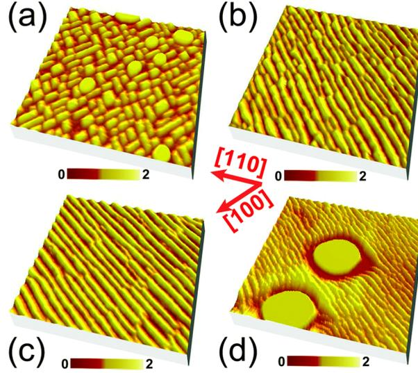
**Figure 1.20:** AFM images ( $0.5 \times 0.5 \mu m^2$ ) of the surface morphologies: (a) 6 ML Ge deposition at 540 °C on Si (001)/[100] 0°; (b) 5.4 ML Ge deposition at 540 °C on Si (001)/[100] 7°; (c) 5.4 ML Ge deposition at 540 °C with a subsequent in-situ annealing for two hours on Si (001)/[100] 7°; (d) 5.4 ML Ge deposition at 650 °C on Si (001)/[100] 7°. The unit of color bar is nm.[33]
