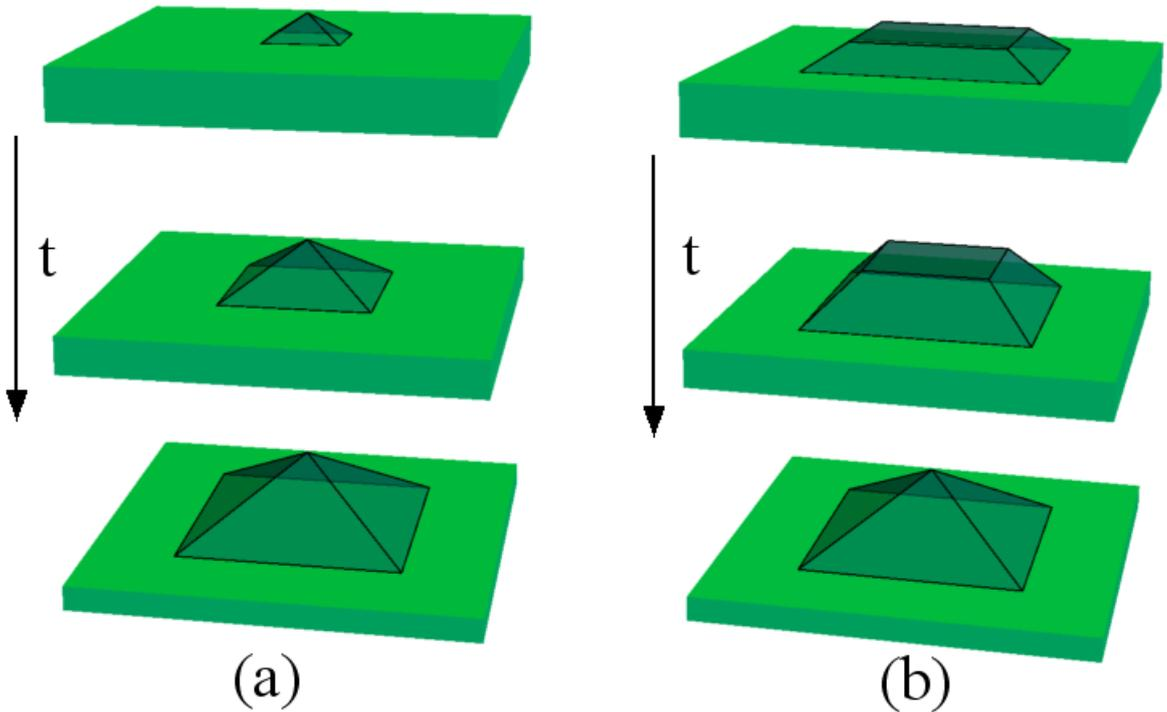
**Figure 2.8:** Two different pathways of pyramidal island nucleation:(a) full pyramid pathway, the island is always (105)-faceted (b) truncated pyramid pathway, the base length is obtained by computing the  $V^*$  of pathway (a) and island grows by stacking materials with (105) facets on sides.
