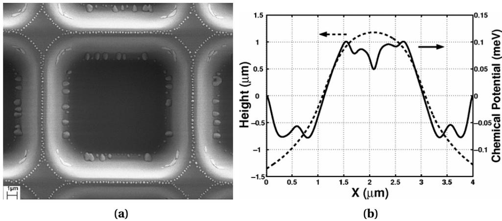
**Figure 1.23:** (a) Scanning electron microscope image of Ge 3D islands ordered on patterned stripes on Si (001) with  $Ge = 60$  MLs. The stripes are oriented in  $\langle 110 \rangle$  directions, but ordering of Ge QDs is independent of this direction. (b) variation of the local surface chemical potential of stripe structures with position  $X$  (solid line). The dashed line is the surface profile measured by AFM[38].
