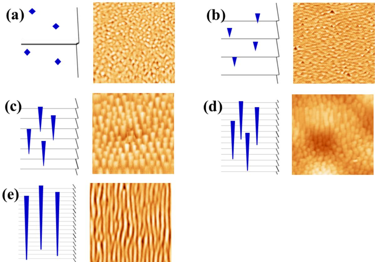
**Figure 4.4:** Evolutions of the correlation length in  $x$  and  $y$  directions (in the plane of the substrate) with the misorientation angle, (a)  $0^\circ$  (b)  $4^\circ$  (c)  $6^\circ$  (d)  $8^\circ$  (e)  $10^\circ$ , with schematic representation of substrate on the left and the corresponding AFM images on the right. The epilayer is  $\text{Si}_{1-x}\text{Ge}_x$  with  $x = 0.22$ .
