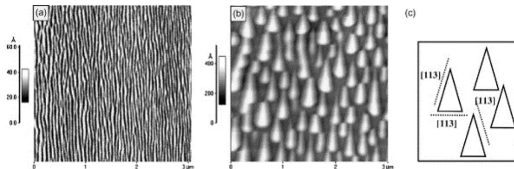
**Figure 1.19:** AFM image ( $3 \times 3 \mu m^2$ ) of  $Si_{0.7}Ge_{0.3}$  islands obtained for a deposited thickness of 10 nm: (a) as-grown; (b) 18 h anneal; (c) is a schematic representation of (113) facets on the annealed sample.[32]
