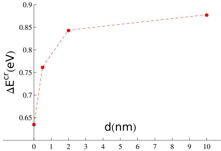
**Figure 3.14:** In case that the strain-dependent surface energy curve is modified, the nucleation energy barrier of forming pyramid as a function of its distance away from an existing pyramid.
