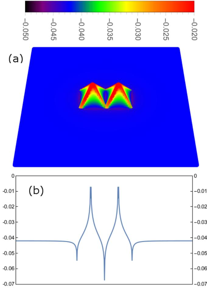
**Figure 3.6:** (a), The distribution of biaxial strain  $\epsilon(\mathbf{r})$  is plotted in case of two touching pyramids ( $d = 0$ ), the value of  $\epsilon(\mathbf{r})$  is represented using colors with scale bar atop; (b), the profile of  $\epsilon(\mathbf{r})$  along the two vertices of pyramid, clearly showing the relaxation on pyramids and strain enrichment around the base of pyramids.
