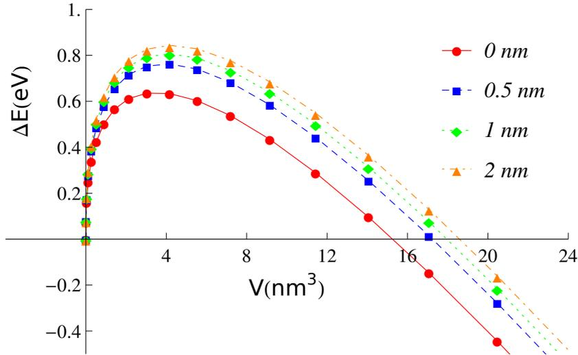
**Figure 3.13:** In case that the strain-dependent surface energy curve is modified, the energy variation  $\Delta E^{total}$  as a function of  $V$  of PB while varying the distance  $d$  from PA, marked as different colors, red, green, blue and yellow respectively for  $d = 0$  nm,  $d = 0.5$  nm,  $d = 2$  nm and  $d = 8$  nm.
