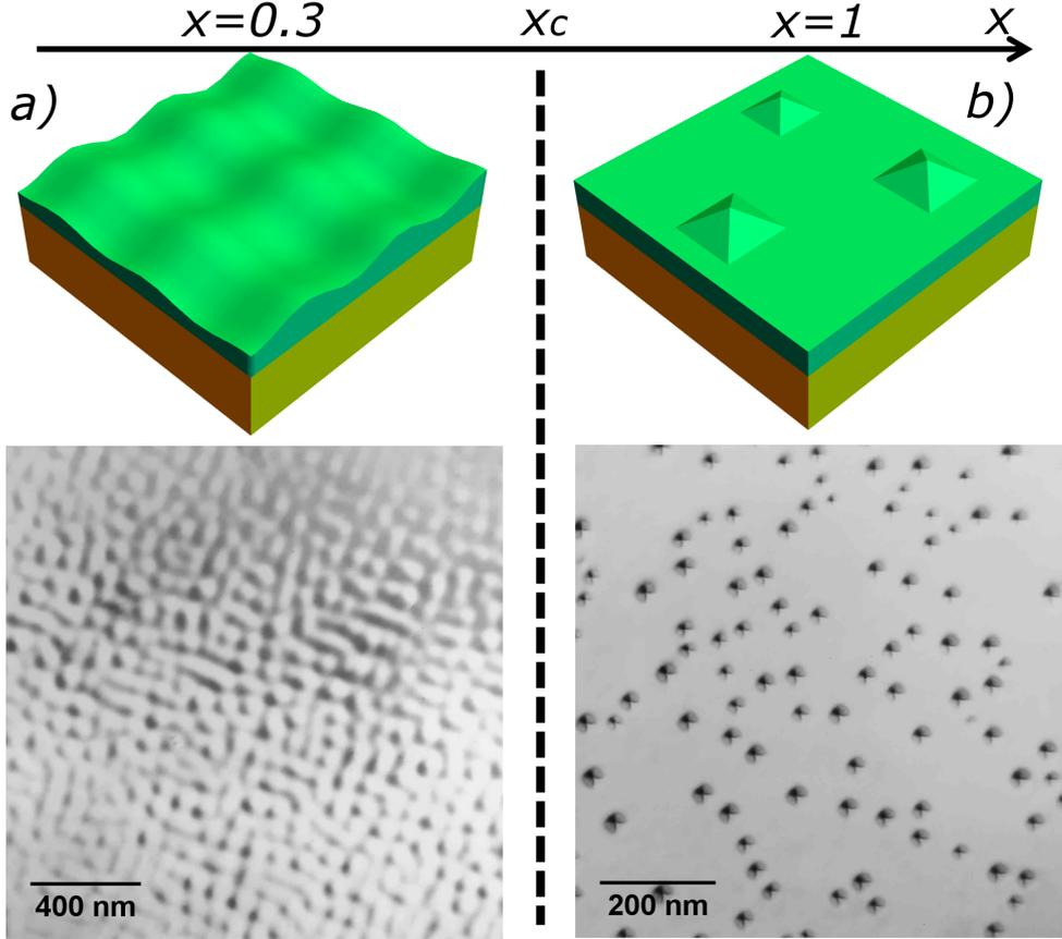
**Figure 2.1:** Growth pathways of  $\text{Si}_{1-x}\text{Ge}_x$  strained layers depending on  $x$ : (a), schematic figure of ATG instability and plan-view TEM image of  $\text{Si}_{0.7}\text{Ge}_{0.3}$  layer ; (b), schematic figure of nucleation and plan-view TEM image of Ge layer.
