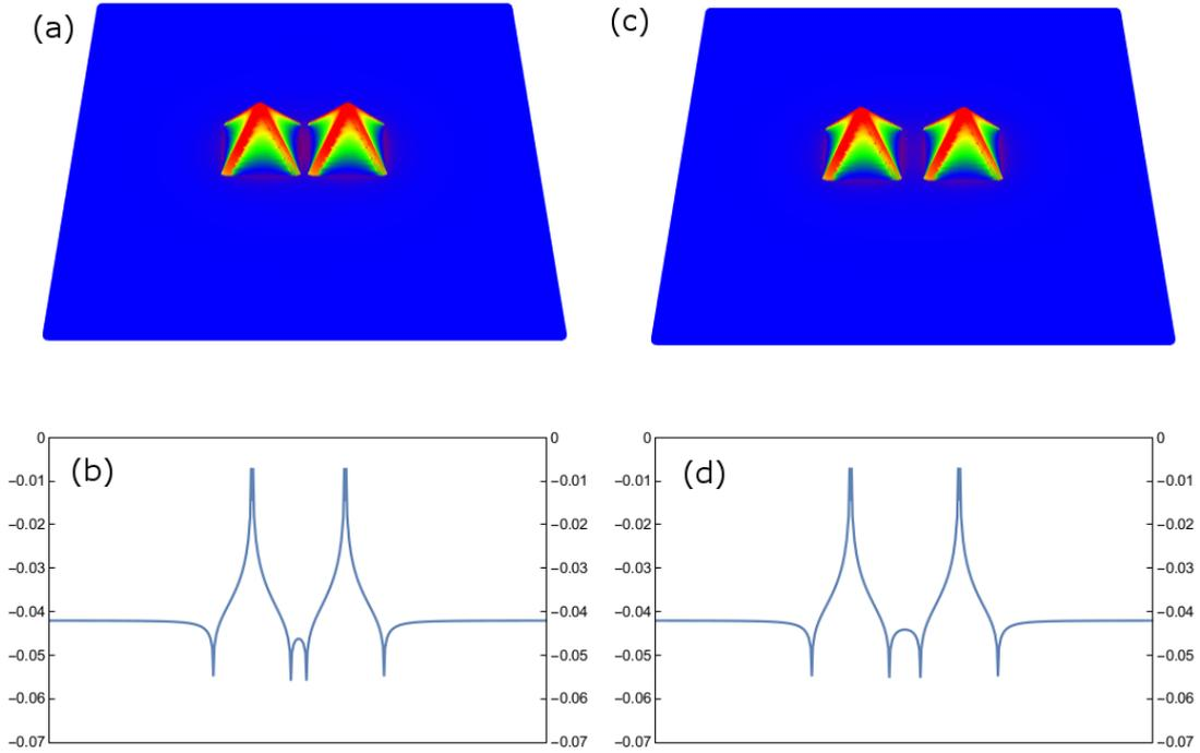
**Figure 3.7:** (a) and (c), The distribution of biaxial strain  $\epsilon(\mathbf{r})$  is plotted for  $d = 2$  nm and  $d = 4$  nm respectively, with the same color scale bar as in Figure 3.6 ; (b) and (d), are the profiles of  $\epsilon(\mathbf{r})$  along two vertexes of pyramid.
