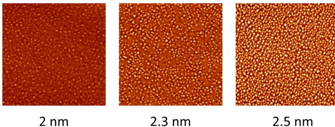
**Figure 5.5:** AFM images of a  $2 \times 2 \mu\text{m}^2$  area of the surface of 2, 2.3, or 2.5 nm thick  $\text{Si}_{0.5}\text{Ge}_{0.5}$  layers which were epitaxially deposited on silicon at 550 °C.
