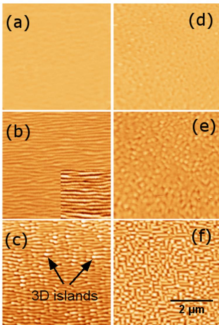
**Figure 4.1:** AFM images of SiGe layers with  $x = 0.22$  and with thickness  $h_{SiGe} =$  (a)–(d) 5 nm, (b)–(e) 8 nm, (c)–(f) 10 nm. For clarity, the vertical scale of all the images is 20 nm.
