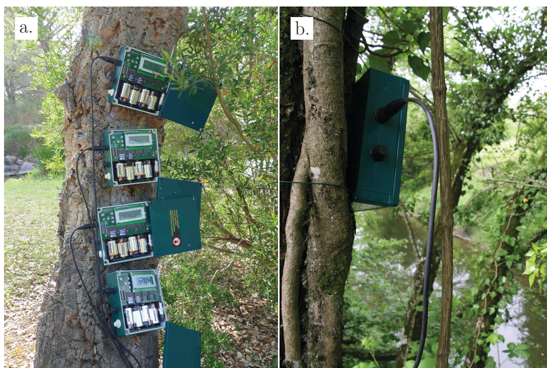
Figure 11 – SM2 autonomous recorders installed in the field. The green boxes contain the autonomous recorders and are connected with a water-proof plug to a hydrophone. a. Four SM2 recorders (cases opened) used to record a Mediterranean pond. b. One SM2 installed in a secondary channel of the river Rhône in Brégnier-Cordon (picture: Diego Llusia).
