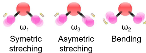
Fig. 2.3 Examples of three vibrational modes of water ( H_2O ) (with the courtesy of Michaël Scherman, ON-ERA/DMPH).
