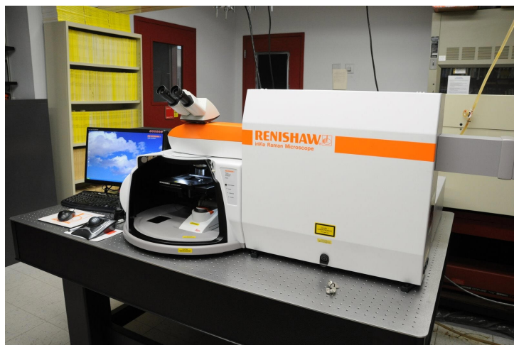
Fig. 2.7 Example of commercially available Raman equipment: Renishaw - inVia Raman Microscope. From http://sciences.usca.edu/chemistry/chad/instrumentation.htm .
