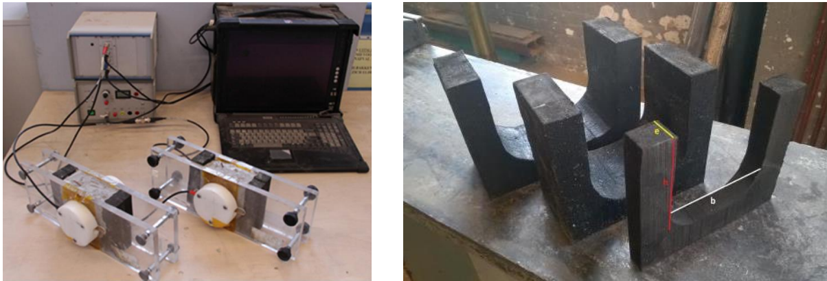
Figure 6 – FreshCon system and mould used for cement paste, mortar and concrete.
