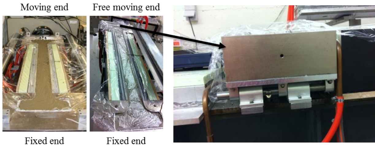
Figure 24 – Left to right: Mould (boundary conditions) – dummy mould (free moving end thanks to ball bearings).
