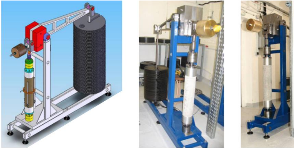
Figure 30 – Uniaxial tensile creep rig with lever arm at Ifsttar [61]
