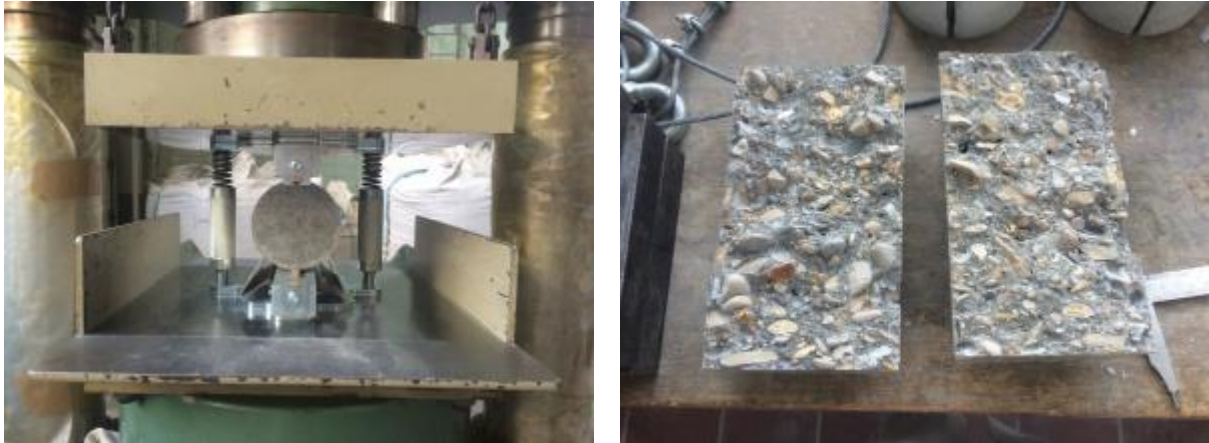
Figure 3 – Splitting tensile test on the Vercors concrete.
