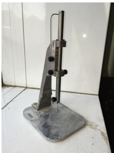
Figure 2 – The Vicat apparatus (left). Evolution of the needle penetration (right)
