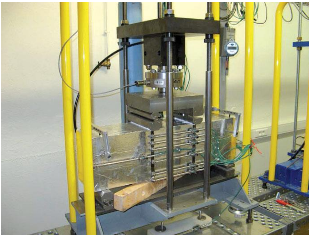
Figure 32 – 4 points bending creep device at Ifsttar [69]
