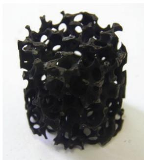
Figure 5.5: Photograph of a SiSiC foam coated with NiRh/MgAl<sub>2</sub>O<sub>4</sub> catalyst after ATR of model biogas
