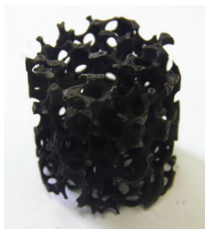
Figure 5.5: Photograph of a SiSiC foam coated with NiRh/MgAl 2 O 4 catalyst after ATR of model biogas
