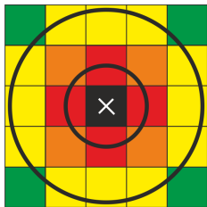
Figure 4.20: Sampling problem when converting the measured image from Cartesian coordinates into polar coordinates.
