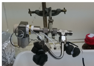
Figure 5.8: Picture of the solid source with sample under the pulsed valve
