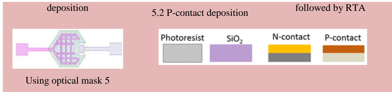
Figure 3.103: Flowchart of phase-5 for p-contact deposition.
