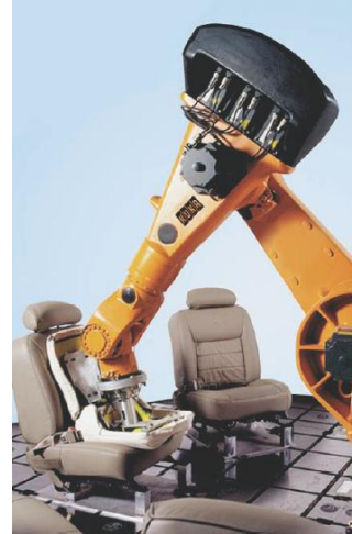
Figure 1.8. – KUKA robot with mass redistribution simplifying its dynamics.
