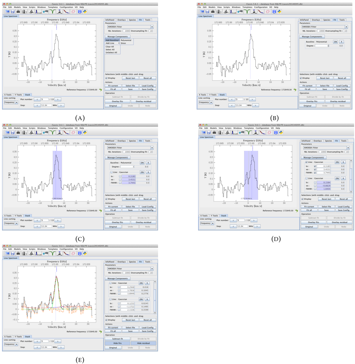
FIGURE 3.8: Snapshot of the CASSIS panel showing the five steps for a two Gaussian fit, with a \text{HC}_3\text{N} line as example.
