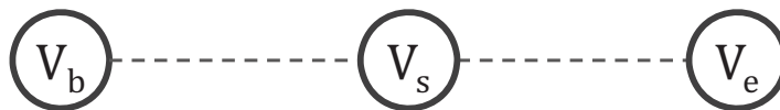
Figure 3.2: A stroke is represented by three vertices in a graph. V_b : begin vertex; V_s : stroke vertex; V_e : end vertex.
