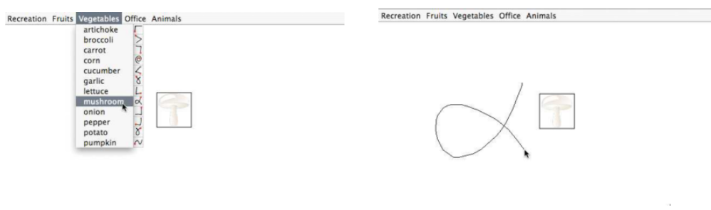
Figure 2.1: Handwritten touch gesture for indirect command: (a) Users may input an icon from the menu. The menu also shows the mapping from strokes to icons. (b) Using stroke as the shortcut to input the icon instead of selecting from menu. [AZ09]
