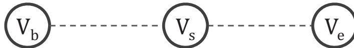
Figure 3.2: A stroke is represented by three vertices in a graph. V_b : begin vertex; V_s : stroke vertex; V_e : end vertex.
