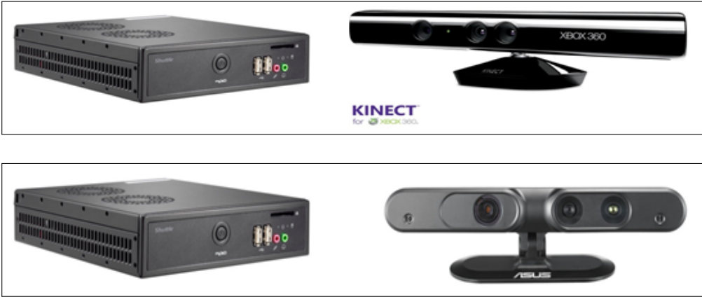
Figure 4.5 – A desktop (running in Windows OS) and Kinect sensor (Figure top) is used to implement the support manager, the game controller and the interaction component. Other kit(desktop running in Linux Fedora 14) (Figure below) is used to implement the recognition component.
