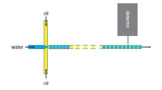
Figure 2.16: Droplet indexing: direct readout. After generation, the droplets flows in the outlet channel until they cross the detector
