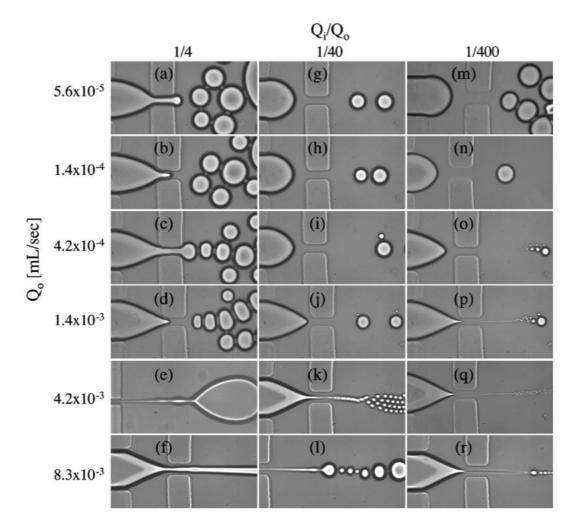
Figure 2.3: Range of droplet size according to the ratio of flow rates of the continuous phase  $(Q_i)$  and dispersed phase  $(Q_o)$ . Reproduction from [61]
