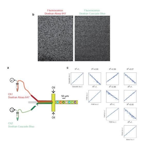
Figure 2.17: Molecular barcoding. Droplets are formed from two aqueous channels containing different fluorophores following a line mapping script (a). The pressure ratio in between the two channels (left) leads to a gradient of concentration, thus fluorescence in between the droplets (b). Scatter plots (in arbitrary fluorescence units) showing the correlation of the fluorescence dyes within a single field of view (N= 218 droplets).
