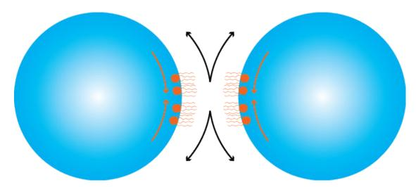
Figure 2.8: Marangoni effect on two approaching droplets: the droplets (blue) are approaching and creates a drainage of the unmiscible phase in between (black arrows) before coalescence. As a result, a Marangoni flow appears on the surface of the droplets (orange arrows) thus concentrating the adsorbed surfactant (orange) on the apex of the droplet. The hydrophobic tails then repel the droplet, stabilizing the emulsion by increasing the drainage time. Adapted from [63]
