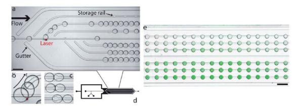
Figure 2.15: Droplet indexing: rail and anchors from Baroud *et al.* [77]. Droplets flow on a central rail (a) until they are deflected to a storage rail by the laser heat (b). Droplets are trapped on the anchor points once the flow is reduced (c), forming a big cluster (d). The flowrate is 40  $\mu$ L.min<sup>-1</sup>. Droplets can be sorted along a gradient of concentration of green fluorescent beads(e). Scale bars are 600  $\mu$ m.
