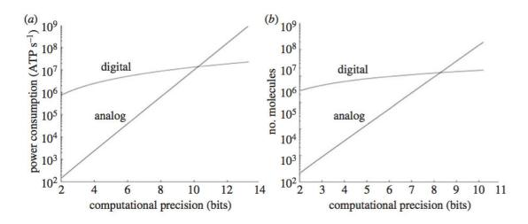
Figure 1.12: Analog versus digital computation in cells. (a) The figure shows the power costs for doing addition in cells with a genetic circuit. (b) The figure shows the molecular protein number required to perform an addition in cells with a genetic circuit. From Sarpeshkar 2014[38]
