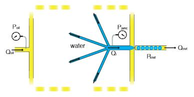
Figure 2.6: Preinjector and nozzle detail: microfluidic parameters.  $P_{oil}$ ,  $Q_{oil}$  are the pressure and flow-rates applied to the oil channels,  $Q_i$  the flow-rate of the aqueous channel,  $P_{junc}$  the pressure in the preinjector,  $Q_{out}$  the flow-rate downstream the junction and  $R_{out}$  the corresponding resistance.
