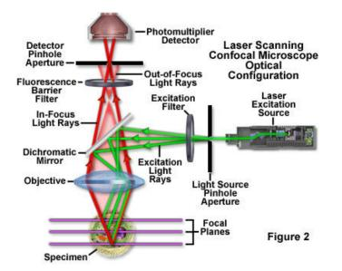
Figure 2.22: Confocal principle in epi-fluorescence laser scanning microscopy, from Olympus Microscopy Ressource Center
