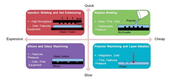
Figure 2.7: Four chip-prototyping methods, from [65].
