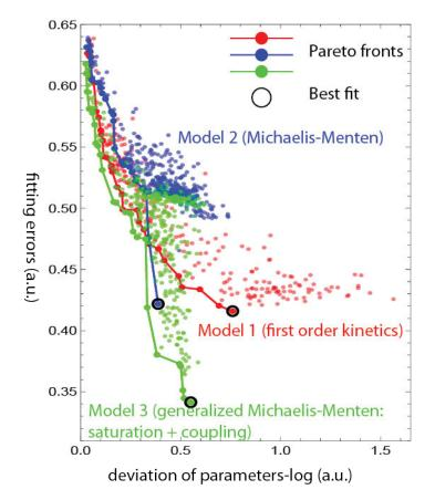
Figure 3.12: Fitting performances of 3 kinetic models. The horizontal axis shows the deviation of the fitted parameters from their initial values. The vertical axis display the distance between the experimental and calculated diagram. Lines represent the pareto fronts for each model, and the best fit is circled in black.
