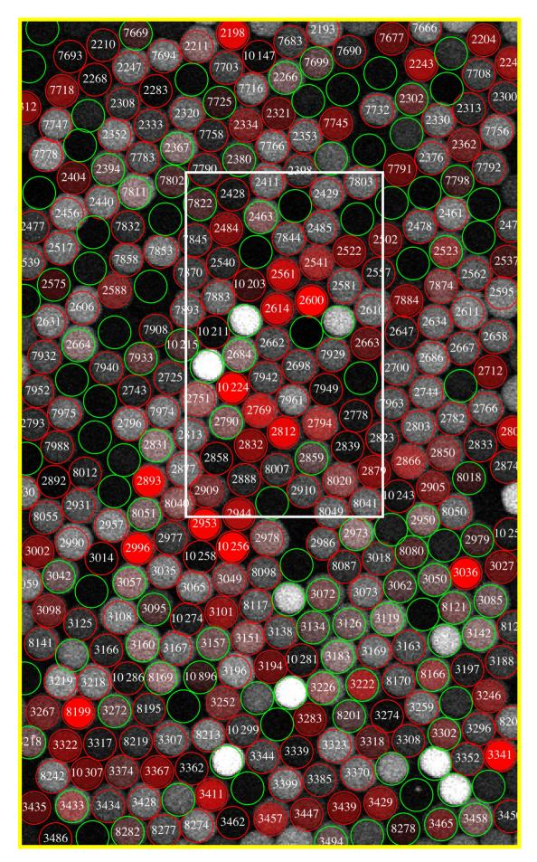
Figure 4.13: Droplet array for the predator-prey system with Bst2.0 WarmStart polymerase. Zoom on the yellow inset in previous image. 368 droplets were detected in this image. 65 of them (circled in green) belong to the self-calibration axes, i.e. they have a ~0 value in one of the three fluorescent barcodes. These are used only during the conversion of barcodes intensities into
