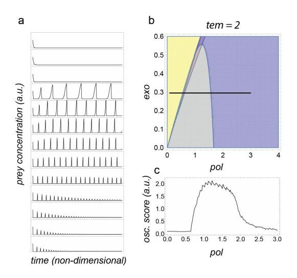
Figure 4.20: **a**, Numerical timetraces for the two-variable model solved with the parameter set  $\{tem = 2, exo = 0.3\}$  and *pol* ranging from .2 (top plot) to 3 (bottom plot) by steps of 0.2 units (corresponding to the black line in the bifurcation diagram shown in **b**. **c**, profile of computed oscillations score for the same segment in parameter space.
