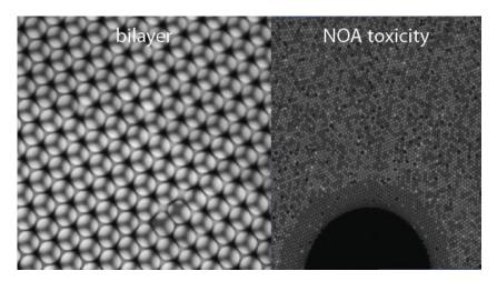
Figure 2.20: Microscopy bloopers: droplets form bilayer (left). Toxicity on the molecular program of photocurable glue NOA81(right).
