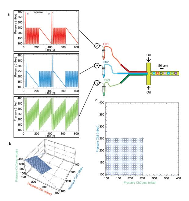
Figure 2.13: Pressure profiles for square mapping. Individual pressures channel by channel (a), square in pressure space with calibration arms (b) and projection in parameter-relevant pressures.
