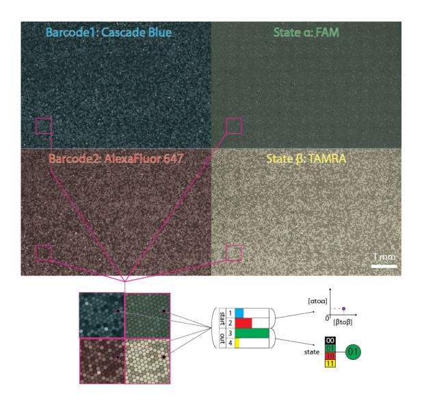
Figure 3.6: Collection of fluorescence levels. For each droplet, we extract the intensities for the barcodes (Cascade Blue and Alexa Fluor 647) and the reporters (FAM and TAMRA). The barcode level gives the initial conditions i.e. the coordinates in the phase space, while the reporter levels render the steady-state of the system. Images show the array after 11h at 42°C.
