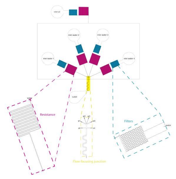
Figure 2.4: Microfluidic circuit developed for the bifurcation diagram mapping. 4 water inlets converge before the nozzle where the oil flow generate the droplets. Highlights: filter area (blue), pre-nozzle serpentine (pink) and post-nozzle serpentine (yellow).
