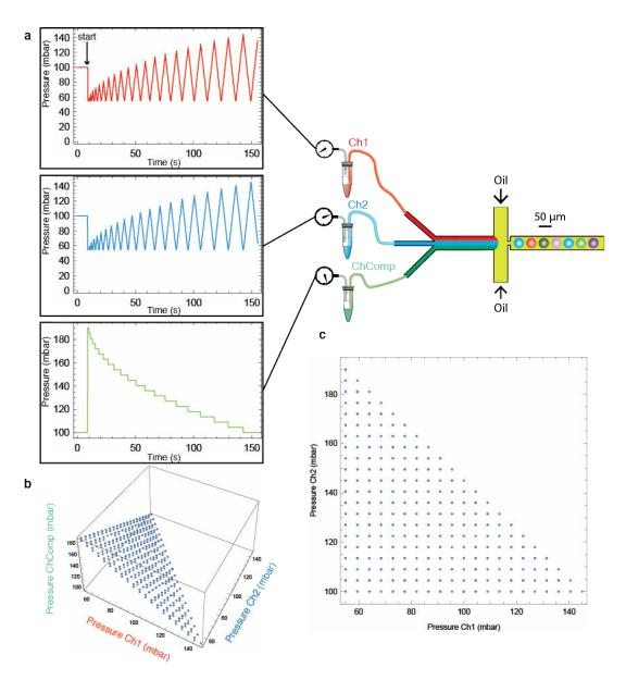
Figure 2.11: Pressure profiles for triangle mapping. for all aqueous channels, the script applies pressures (a) whose sum draws the simplex in pressure space (b). While projected according to the parameter-relevant pressures (i.e. pressures for which the aqueous solution contains a parameter) the shape of the triangle appears (c).
