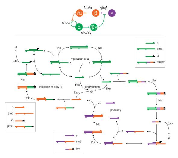
Figure 3.4: Alternative bistable circuit : reactions network and corresponding implementation in PEN-DNA toolbox framework
