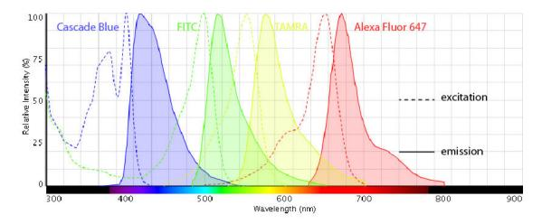
Figure 4.6: Four fluorophores used to map the diagram: Cascade Blue, FITC and Alexa Fluor 647 barcode the parameters, and TAMRA to record the evolution of the system.
