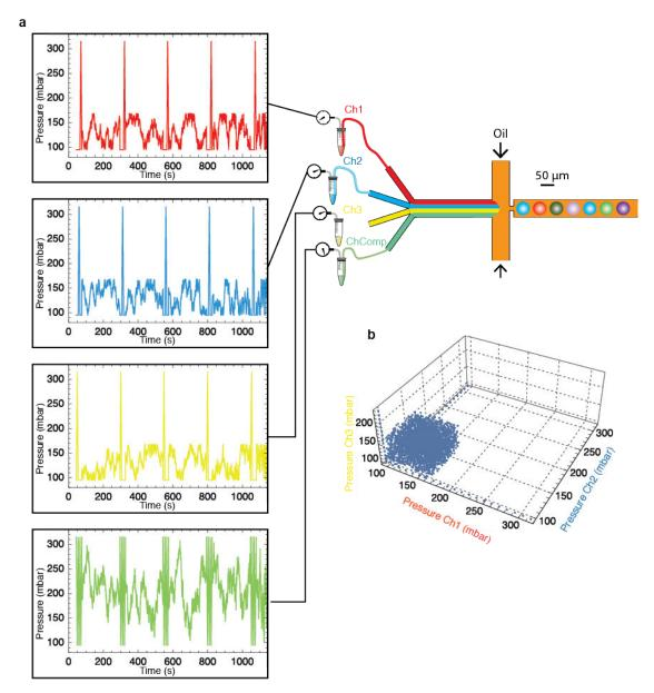
Figure 2.14: Pressure profiles (a) and resulting volume in pressure space (b) for random-walk cube mapping.
