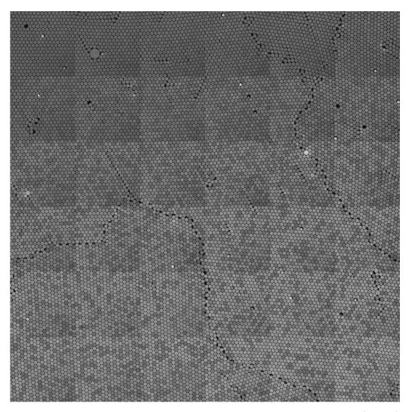
Figure 4.8: Scanning area limitation: first frame of a timelapse. The first images (top left) are homogenous -meaning chemistry did not occurred yet- while the late images show contrast amongst the droplets.
