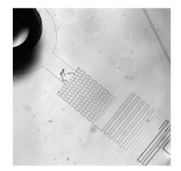
Figure 2.5: Dust from solution/tubing trapped by the filters.
