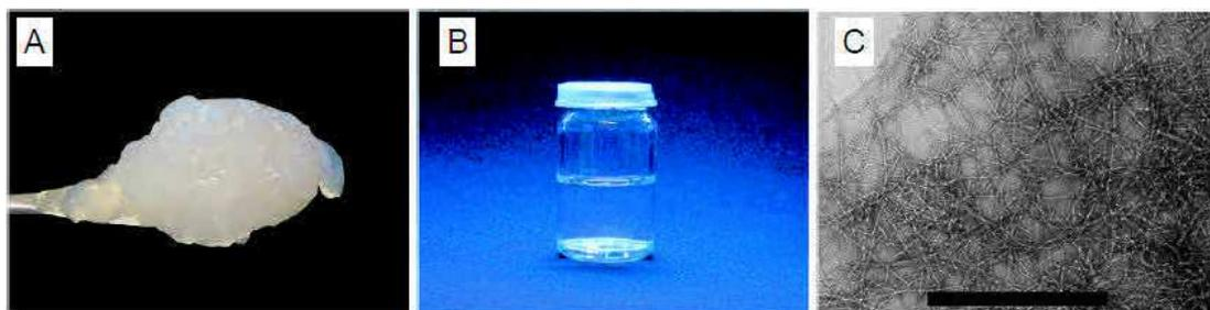
**Figure II-2.** A) Photograph of the viscous and transparent gel pulp formed by the cellulose nanofibrils (images credited to Dr. Rémi Merindol); B) transparent solution of CNFs obtained after the ultrasonication, centrifugation and filtration;<sup>103</sup> C) TEM image of the CNFs solution described in B, the scale bar is 500 nm.<sup>103</sup>
