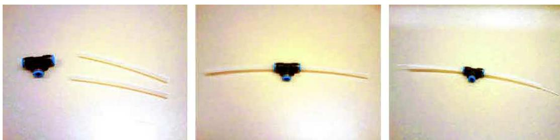
**Figure II-9.** a) Photograph of a t-junction and two 8 mm tubes; b) photograph of the two tubes connected by the t-junction; c) photograph of a single hollow fiber membrane inserted into the two tubes connected by t-junction (images taken by project partner).
