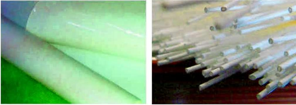
**Figure II-8.** a) Photograph of a typical flat sheet membrane made by non-solvent induced phase separation (NIPS); b) photograph of hollow fiber membranes HF from project partner.
