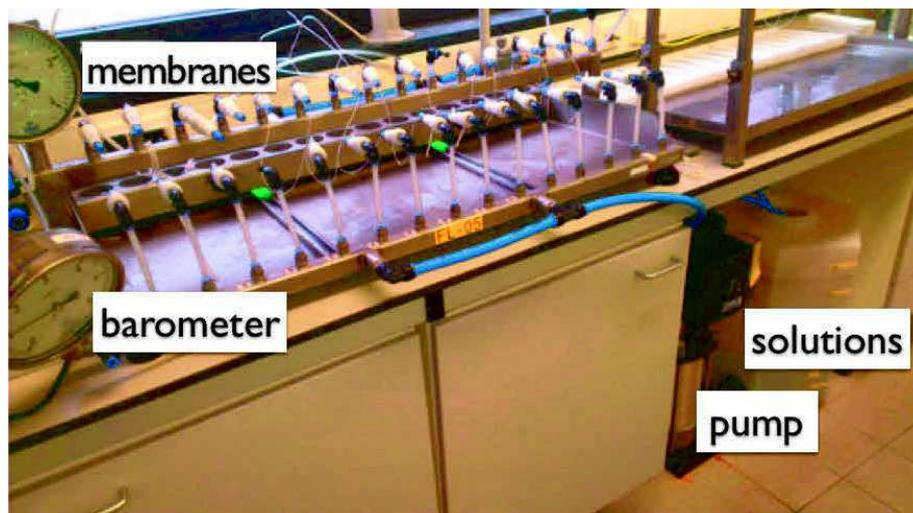
**Figure II-25.** Photograph of a typical set-up for the membrane retention and permeability tests (image from project partner).
