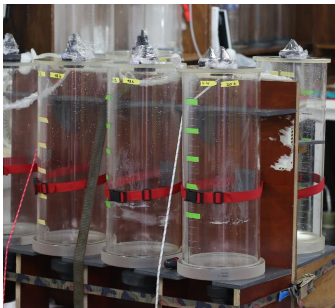
Figure 2.2: Perspex filtrations units used for the determination of Ba_{xs} concentrations during the GEOVIDE cruise
