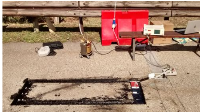
Figure 7.24: Test setup with coil L_5 placed in the hole and covered with liquid bituminous coating.
