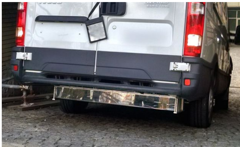
Figure 6.20: Receiver structure mounted under the vehicle.
