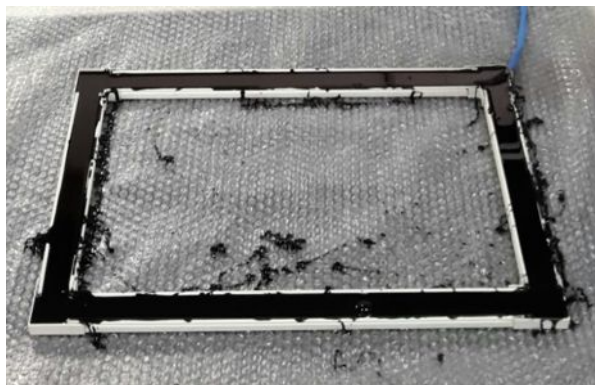
Figure 7.14: Coil B with the plastic wire way filled with bituminous coating.
