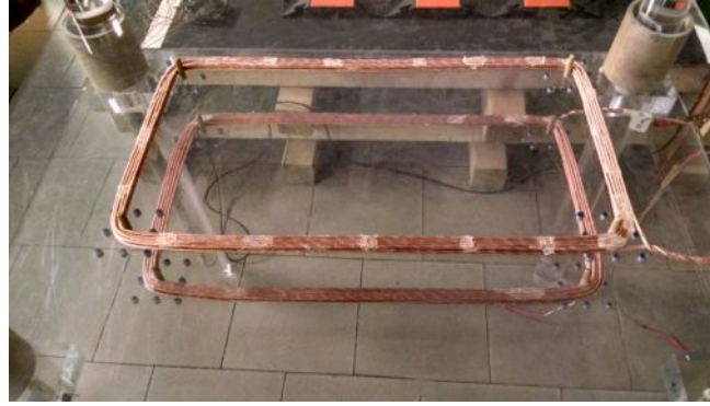
Figure 4.8: IPT prototype for the testing the frequency behaviour.
