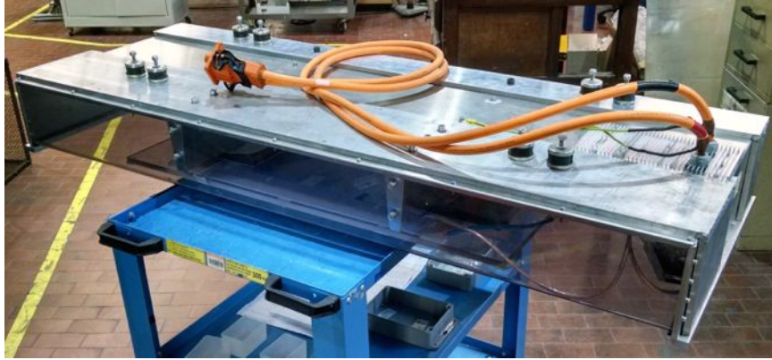
Figure 6.19: Complete receiver structure ready to be mounted under the vehicle.
