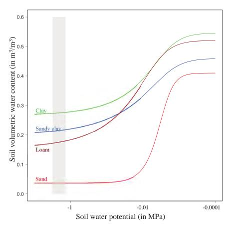
**Fig. 2.** Soil volumetric water content as a function of soil water potential, according to van Genuchten (1980) equation, for four different soil types. Parameters for clay, loam, sand and sandy clay soil are from Hodnett & Tomasella (2002). The grey vertical shaded zone corresponds to the range of leaf water potential at turgor loss point found in Chapter 2 of this thesis (Maréchaux *et al.* 2015).
