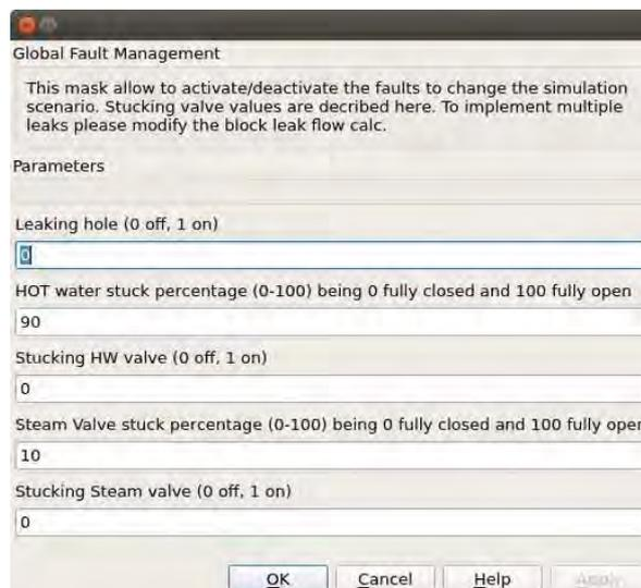
Figure 10.23: Pilot Plant Model Mask. It allows to activate or deactivate the implemented faults for change the simulation scenario.
