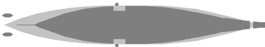
Figure 39 – Parallel waterplanes for  $d=6.00$  m (light grey) and  $d_L=3.33$  m (dark grey).
