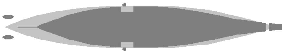
Figure 39 – Parallel waterplanes for d=6.00 m (light grey) and d_L=3.33 m (dark grey).
