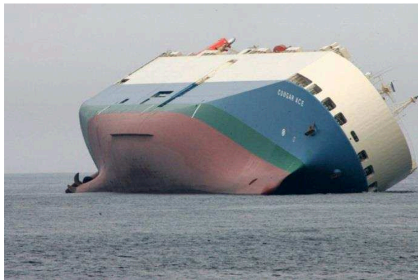
Figure 5 – Pure Car Carrier Cougar Ace with severe heel on port side (photo from National Digital Library of the United States Fish and Wildlife Service).
