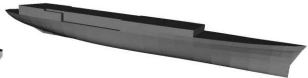
Figure 125 – Watertight volume of the Jeanne d'Arc .
