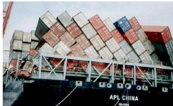
Figure 112 – Damage occurred on the *APL China* after a parametric roll accident in October 1998 (from [afcan.org](http://afcan.org)).
