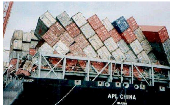
Figure 112 – Damage occurred on the APL China after a parametric roll accident in October 1998 (from afcan.org ).
