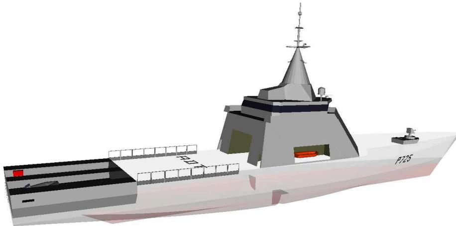
Figure 93 – Superstructures of the Offshore Patrol Vessel *Adroit*.
