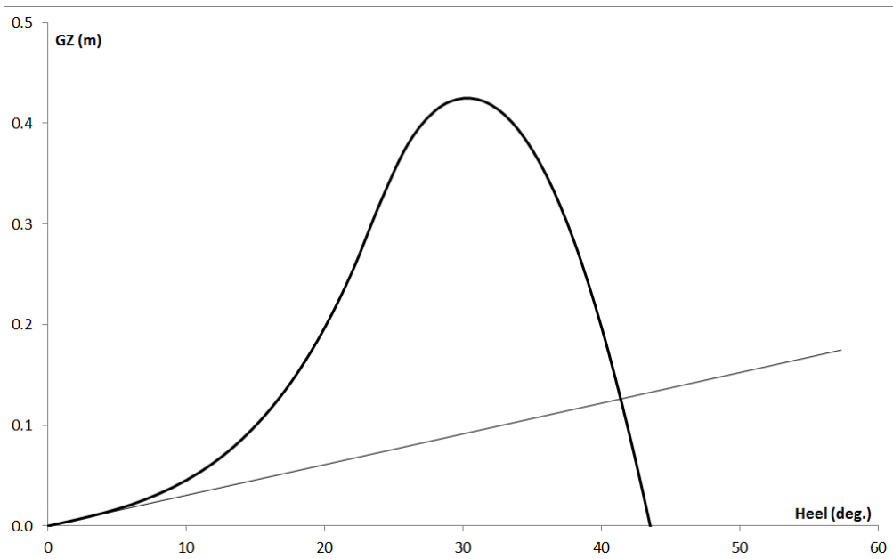
Figure 78 – GZ curve of the tanker at a draft equal to 11 m.
