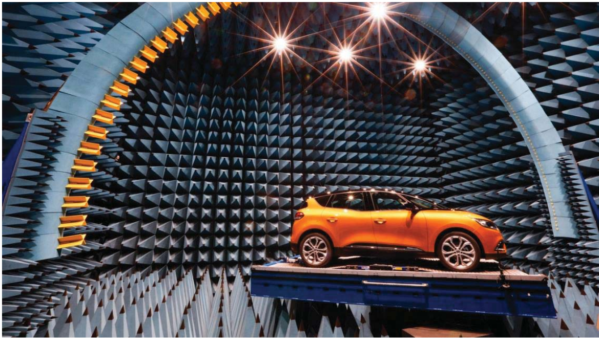
Figure 4-3 : Full anechoic measuring facility
