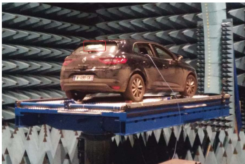
Figure 4-16 : Measuring configuration of a patch antenna on the rear window
