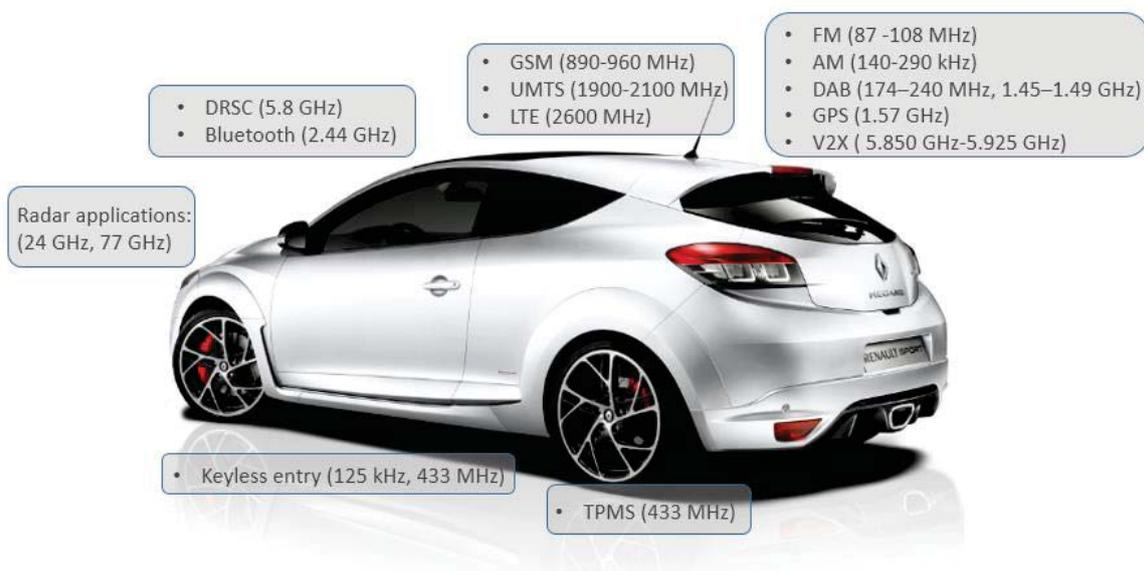
Figure 4-1 : Frequency ranges of the multiple RF automotive services.
