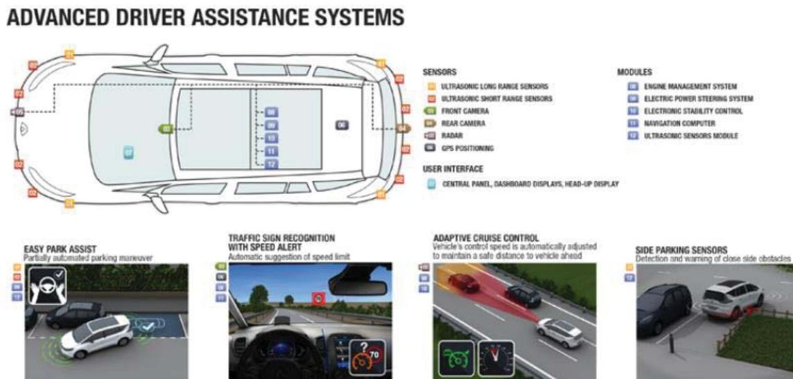
Figure 2-8 : ADAS applications developed by Renault.
