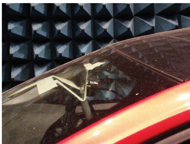
Figure 6-4 : Mounted configuration of the patch antenna on the front windscreen
