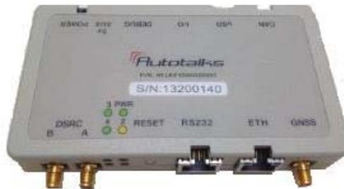
Figure 6-5 : Modem provided by Autotalks used during measurement campaigns
