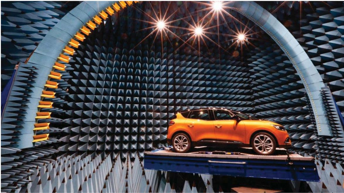
Figure 4-3 : Full anechoic measuring facility
