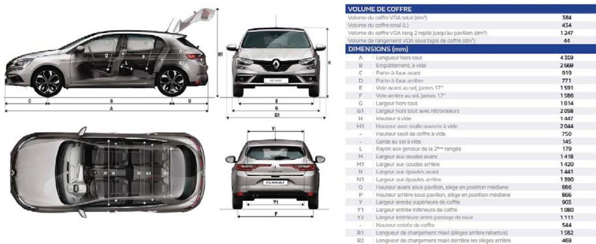
Figure 6-2 : Blueprint and dimensions of the Mégane IV
