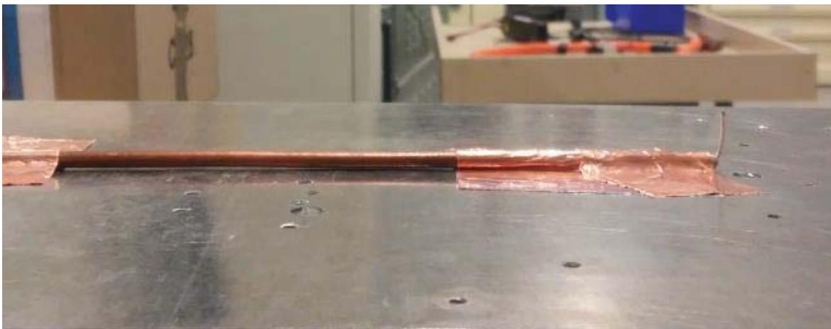
Figure 4-11 : A crafted monopole using a semi-rigid cable
