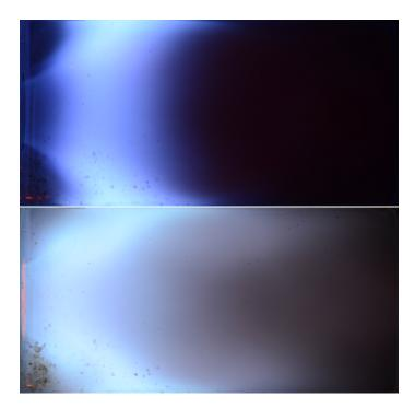
Figure A.13: Flame shape of Op16-0-2 at fully premixed and partially premixed functioning
