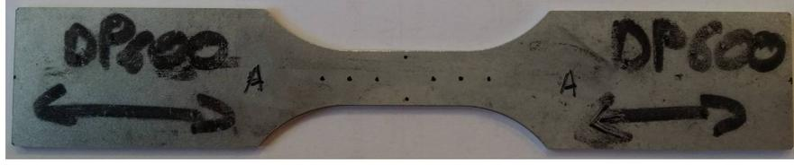
FIGURE 2.3 – The mark points of the tensile specimen
