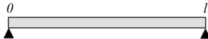
$$\left\{ \begin{array}{l} X(0) = 0 \\ X''(0) = 0 \end{array} \right. \quad \left\{ \begin{array}{l} X(l) = 0 \\ X''(l) = 0 \end{array} \right.$$
