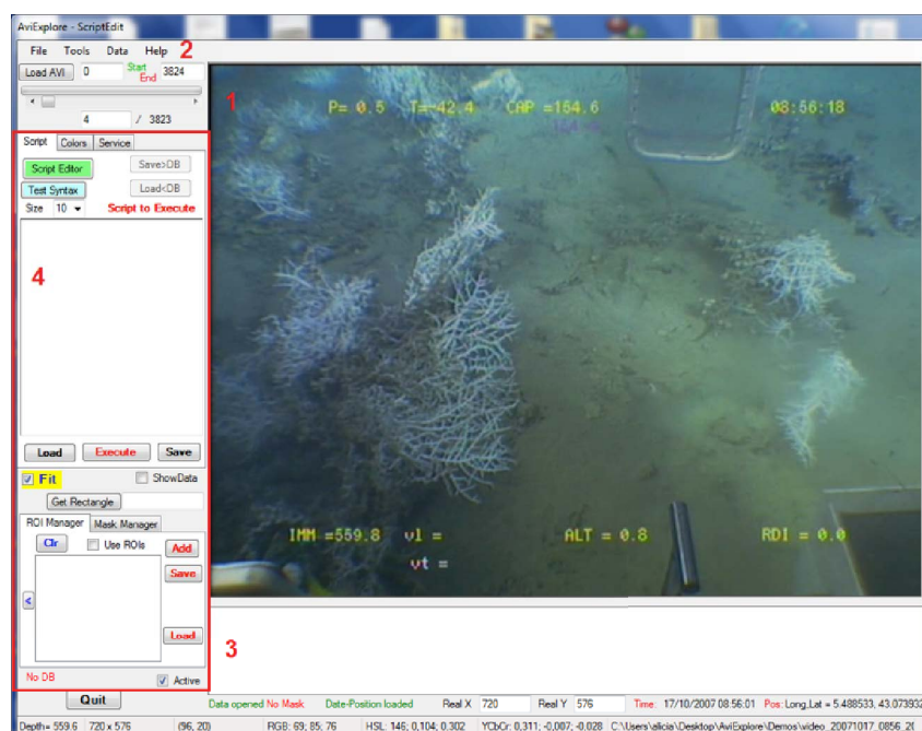
Figure AIV.4 : AVIExplore – Mobile, AVIExplore – Fixed and AVIExplore – ScriptEdit module's general graphic user interface: (1) video display window, (2) strip menu, (3) video time scrollbar, and (4) area differing between modules.
