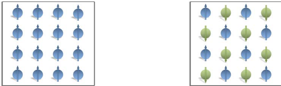
Fig. III.2: Sketches of a ferromagnetic order if J > 0 (on the left-hand side) or an anti-ferromagnetic order with J < 0 (on the right-hand side).
