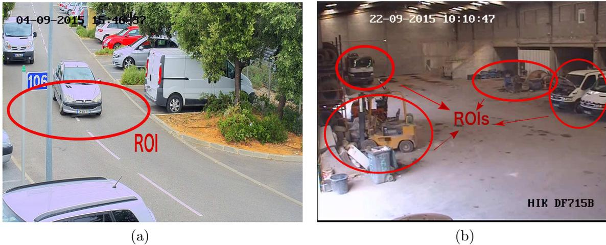
Figure 8.4: This figure shows some Regions of Interests (ROIs) in a picture of video streams captured from 4G-TECHNOLOGY. In picture (a) the receiver is interested in the car number plates while in (b) to the material/equipment in a working area. The retina-inspired codec is able to provide to the receiver some copies of these ROIs with a lower distortion than the parts of the scene which are out of the ROIs.
