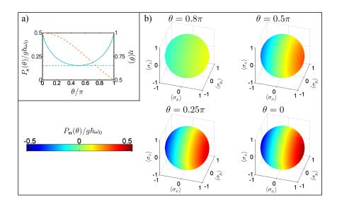
**Figure 1.4** – Performances of the MPE. a) Efficiency  $\eta(\theta)$  (solid blue) and normalized power  $P_{\mathbf{x}}(\theta)/g\hbar\omega_0$  when the working point of the engine is  $|+_{\mathbf{x}}\rangle$ , as a function of the Rabi angle  $\theta$ . b) Normalized power  $P_{\mathbf{n}}(0)/g\hbar\omega_0$  as a function of the working point in the Bloch sphere.
