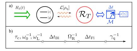
**Figure 3.1** – Timescales of the problem. a) Situation under study: a Qubit is driven by a coherent drive generating the time-dependent term  $H_d(t)$  in its Hamiltonian. The Qubit is coupled to an electromagnetic reservoir assimilated to a thermal reservoir at temperature *T*. b) Relative magnitude of the frequency parameters and of the two possible coarse-graining time steps leading to the FME ( $\Delta t_{Fl}$ ) and to the OBEs ( $\Delta t_{Bl}$ ).
