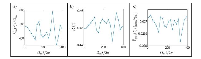
**Figure 4.6** – Scattering at long time-scale. Internal energy  $\bar{U}_{m}(t)$  of the MO (a), Qubit population  $\bar{P}_{e}(t)$  (b) and heating rate  $\bar{\Gamma}_{opt}(t)$  (c) averaged over 20 mechanical periods.
