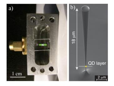
**Figure 2** – Experimental platforms. a) Superconducting circuit implementing a quantum electrodynamics experiment, involving a Qubit dispersively coupled to a cavity. Picture from the Quantum Electronics Group of Ecole Normale Supérieure (Paris, France). b) Hybrid optomechanical setup featuring a quantum dot (Qubit) embedded in a vibrating nanowire. Picture from the NanoPhysics and SemiConductors team of the the Institut Néel - CNRS and CEA (Grenoble, France).
